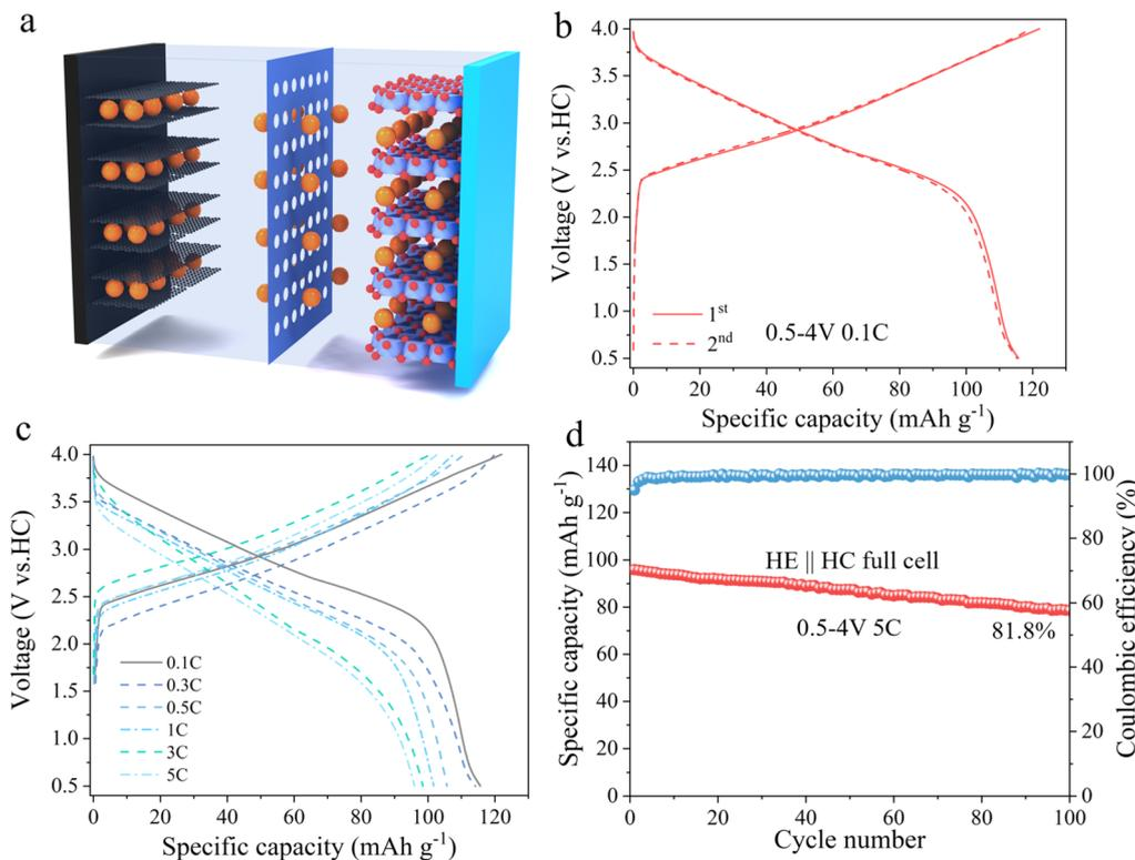
**Fig. 6** Electrochemical performance of HE full cell. (a) Schematic diagram of the full cell. (b) Charge–discharge curves of the material at 0.1C current density in the voltage range of 0.5–4 V. (c) Electrochemical curves of the material at different current densities. (d) Cycling plot of HE for 100 cycles under 5C conditions.
