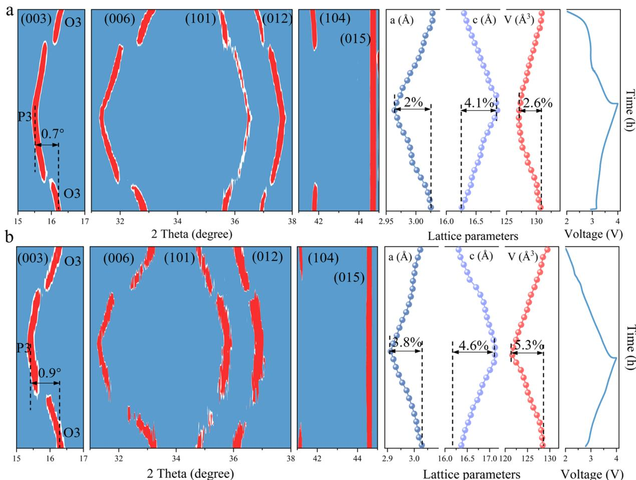
Fig. 5 The structural evolution during Na<sup>+</sup> extraction/insertion. (a) The phase transition process of HE and the variation of lattice constants. (b) The phase transition process of NFM and the variation of lattice constants.
