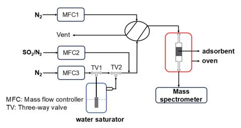
Fig. 1 Schematic of the column breakthrough setup.
