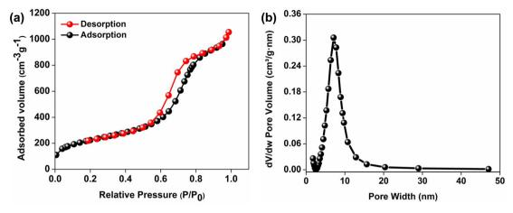
Fig. 2 (a) N<sub>2</sub> adsorption–desorption isotherm and (b) pore size distribution of PE-AlSiO<sub>2</sub>.
