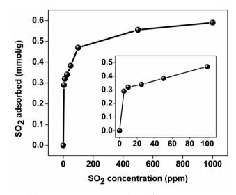
Fig. 5 SO<sub>2</sub> adsorption isotherms of GD-PEI/S.
