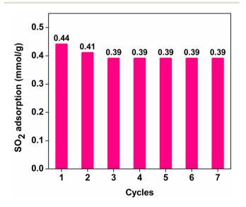
Fig. 7 Regeneration cycles of GD-PEI/S under dry 100 ppm  ${\rm SO}_2$  balance  ${\rm N}_2$ .
