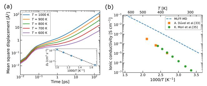
Fig. 6 (a) Mean square displacement (MSD) as a function of time and (b) ionic conductivity as a function of 1000/T, for F atoms in  $Ba_{0.5}Ca_{0.5}F_2$ . In the inset of (a), diffusion coefficients ( $D_F$ ) obtained by fitting the MSDs are plotted. In (b), the experimental values for Ba<sub>1-x</sub>Ca<sub>x</sub>F<sub>2</sub> with  $x \sim 0.5$  (ref. 33 and 35) are plotted for comparison.
