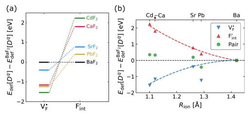
Fig. 9 (a) Comparison of the relative formation energies of  $V_F^*$  and  $F_{int}'$  of  $AF_2$  (A=Ca, Ba, Sr, Cd, Pb) with regard to  $BaF_2$  and (b) its dependence on the ionic radius of A<sup>2+</sup> with eight coordination.<sup>76</sup> In (b), points for half the formation energies of the anion Frenkel pair and fitted lines with a parabolic function except for PbF<sub>2</sub> for guiding eyes are also shown.
