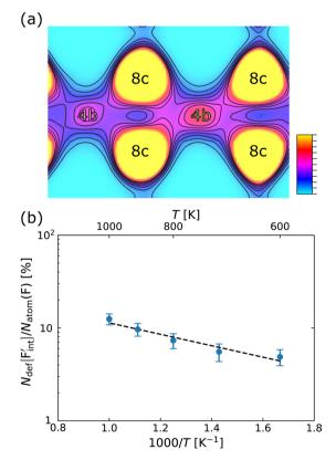
Fig. 7 (a) Distribution of F-atoms on the (110) plane at T=1000 K, where F-atom trajectories in the supercell are contracted into a unit conventional cell. (b) Extracted and averaged existence probability of F-atoms on the interstitial sites
