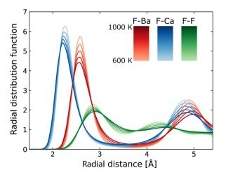
Fig. 5 Radial distribution functions around F atoms in Ba<sub>0.5</sub>Ca<sub>0.5</sub>F<sub>2</sub>.
