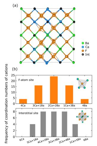
Fig. 2 (a) Relaxed SQS structure in the 2  $\times$  2  $\times$  2 conventional supercell of Ba<sub>0.5</sub>Ca<sub>0.5</sub>F<sub>2</sub> and (b) histogram of the combination of coordinating cations around the F-atom sites (8c) and interstitial sites (4b) in the fluorite supercell.
