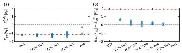
Fig. 11 Point-defect formation energies of (a) F-vacancies and (b) interstitial F-atoms in  $Ba_{0.5}Ca_{0.5}F_2$ , which is measured from the values in  $BaF_2$ . The red dotted lines indicate the corresponding energies for  $CaF_2$ .
