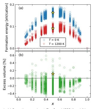
Fig. 1 (a) Formation energies at T=0 and 1200 K and (b) excess volume of  $Ba_{1-x}Ca_xF_2$  solid solution as a function of composition, x. The yellow star symbols indicate the values of the SQS model with a 2  $\times$  2  $\times$  2 conventional supercell.
