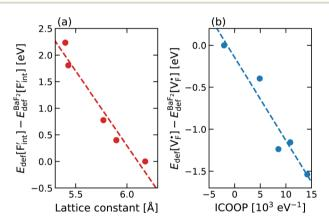
Fig. 10 Correlation plots of relative defect formation energies for (a) interstitial Fions and (b) F-ion vacancies for AF<sub>2</sub> (A = Ca, Ba, Sr, Cd, Pb). For the descriptors, see the main text.
