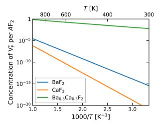
Fig. 4 Point-defect concentrations as a function of temperature, where  $\mu_F$  is fixed to be the value for Cu/CuF<sub>2</sub>. Under these conditions, anion Frenkel pairs are dominant.
