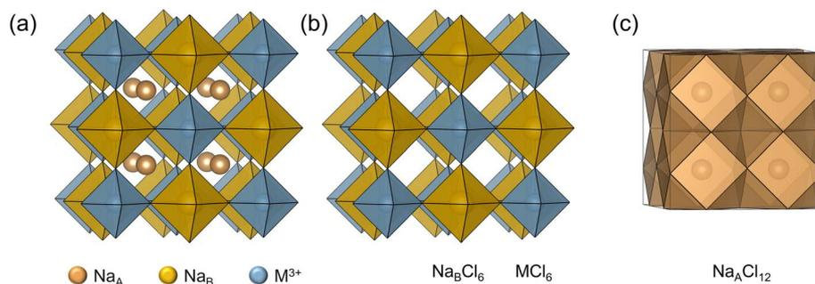
Fig. 1 Ideal non-distorted  $\text{Na}_3\text{MCl}_6$  perovskite crystal structure (hypothetical). (a) Full structure. (b) The building units of  $\text{Na}_B\text{Cl}_6$  and  $\text{MCl}_6$  octahedra. (c) The building units of  $\text{Na}_A\text{Cl}_{12}$ .
