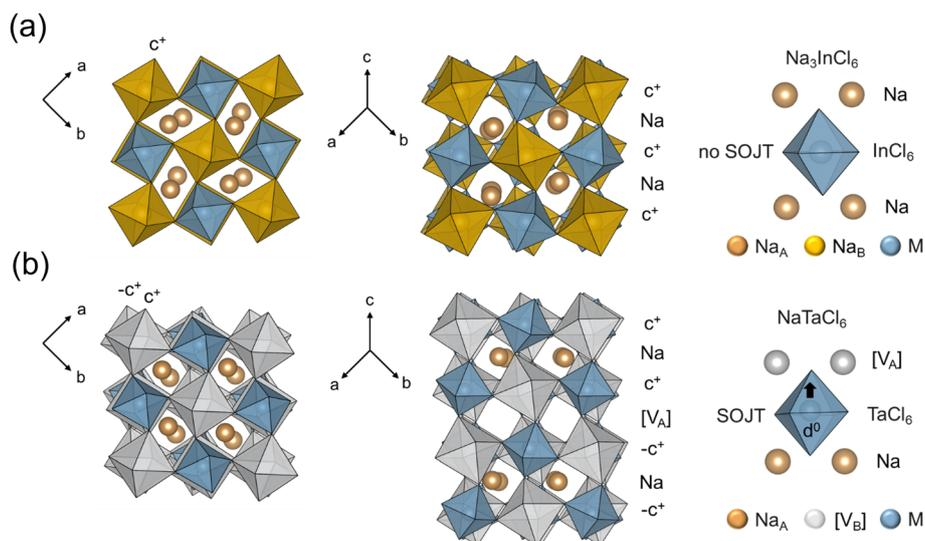
Fig. 4 Crystal structure comparison of  $\text{Na}_3\text{InCl}_6$  and  $\text{NaTaCl}_6$ . Most representative projections of the crystal structure of (a)  $\text{Na}_3\text{InCl}_6$  and (b)  $\text{NaTaCl}_6$ .
