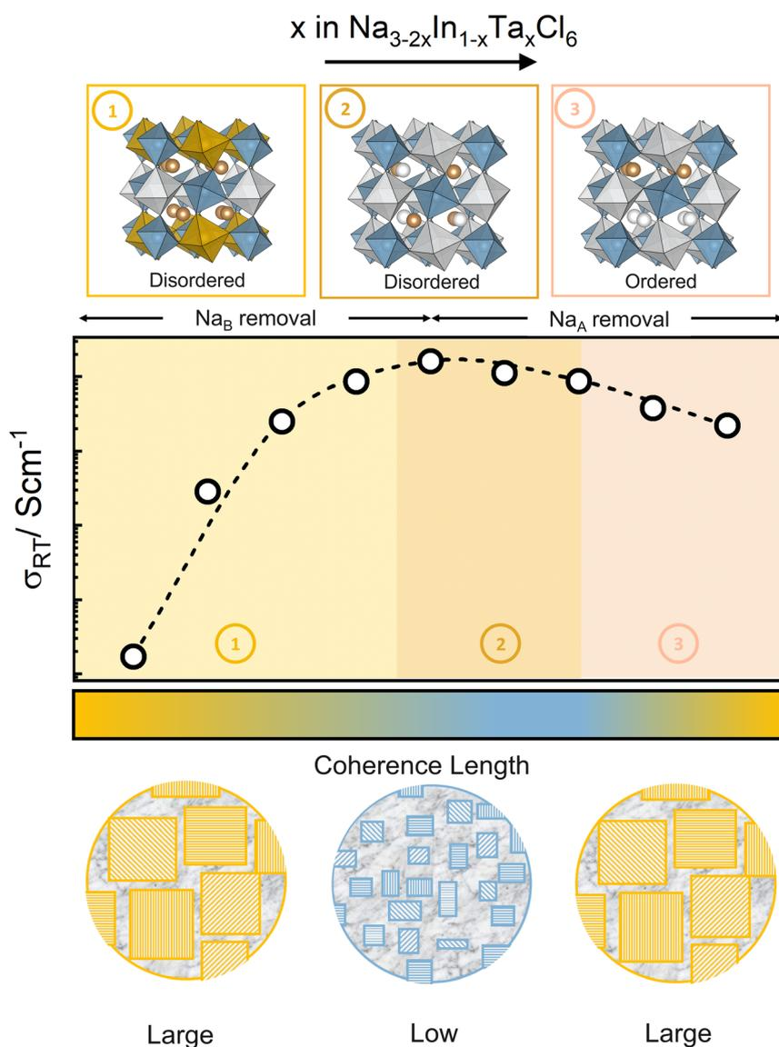
Fig. 9 Crystal structure – microstructure – ionic transport coupling. Schematic of perovskite crystal structures illustrating the three different  $\text{Na}^+$  vacancy arrangements as function of the Na vacancy content. The different stages correlate with the coherence length and the ionic transport properties trends. Schematic of samples with large (yellow) and (small) coherence is also shown.
