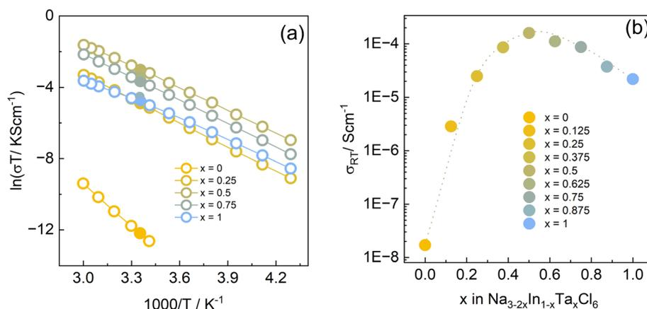
Fig. 6 Ionic transport of  $\text{Na}_{3-2x}\text{In}_{1-x}\text{Ta}_x\text{Cl}_6$ . (a) Arrhenius plot of the ionic conductivity as a function of temperature for some members of  $\text{Na}_{3-2x}\text{In}_{1-x}\text{Ta}_x\text{Cl}_6$  ( $x = 0, 0.25, 0.5, 0.75$  and 1). Filled circles are indicating the values at room temperature. (b) Room temperature ionic conductivity evolution in  $\text{Na}_{3-2x}\text{In}_{1-x}\text{Ta}_x\text{Cl}_6$ .
