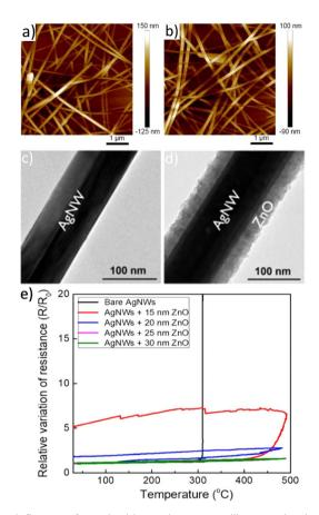
Fig. 4 Influence of metal oxide coating on metallic nanowires in terms of roughness and stability. AFM image of (a) AgNW network deposited on a glass substrate, (b) spin-coated TiO2 films on top of AgNW network. TEM images of (c) bare pristine AgNW, (d) AgNW coated with a 30 nm thick ZnO, deposited by SALD. Normalized resistance (e) during thermal stress of bare AgNW network and coated with different ZnO thickness. Reproduced with permission from American Chemical Society. 165,166
