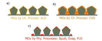
Fig. 3 Main features related to the coating of metallic nanowires depending on the coating process. Metal oxides (MOx) homogeneity, surface coverage, and conformality on the silver nanowires depending on the method employed, namely (Ch.) chemical processes (a) ALD, (b) CVD, and (Phys.) physical processes (c) Sputt, Evap, and PLD.
