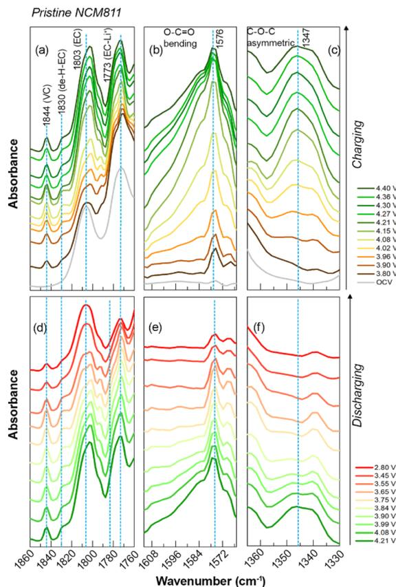
Fig. 1 Operando FTIR spectra of pristine NCM811 during (a–c) charging and (d–f) discharging. VC is present at  $1844\text{ cm}^{-1}$ , de-H EC at  $1830\text{ cm}^{-1}$ , and O–C=O bending vibration at  $1573\text{ cm}^{-1}$ . The C–O–C asymmetric stretching vibration is present at  $1347\text{ cm}^{-1}$ .
