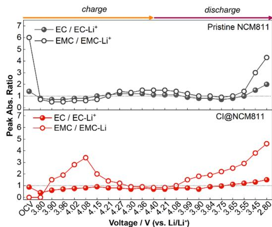
Fig. 6  $\text{Li}^+$  solvation behavior comparison of (a) pristine NCM811 and (b) CI@NCM811 represented by a ratio of EC/EC- $\text{Li}^+$  and EMC/EMC- $\text{Li}^+$ . EC is present at  $1806\text{ cm}^{-1}$ , EC- $\text{Li}^+$  at  $1773\text{ cm}^{-1}$ , EMC at  $1747\text{ cm}^{-1}$ , and EMC- $\text{Li}^+$  at  $1717\text{ cm}^{-1}$ .
