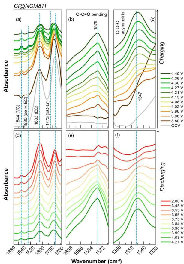
Fig. 3 Operando FTIR spectra of CI@NCM811 during (a-c) charging and (d-f) discharging. The VC presents at 1844  $\text{cm}^{-1}$ , de-H EC presents at 1830  $\text{cm}^{-1}$ , and O=C=O bending vibration presents at 1573  $\text{cm}^{-1}$ . The C-O-C asymmetric stretching vibration presents at 1347  $\text{cm}^{-1}$ .
