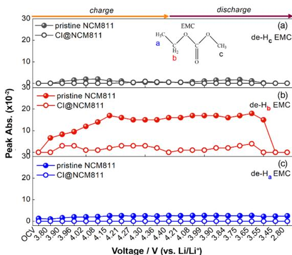
Fig. 5 Peak assignment behavior of pristine NCM811 and CI@NCM811 represented by the absorption intensity of (a) de-H<sub>e</sub> EMC at 1741  $\text{cm}^{-1}$ , (b) de-H<sub>e</sub> EMC at 1751  $\text{cm}^{-1}$ , and (c) de-H<sub>a</sub> EMC at 1761  $\text{cm}^{-1}$ .
