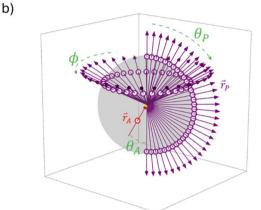
Fig. 7 (a) Vector representations of the transition dipole moments of A (red) and PX (purple) with the chromophore centroid depicted as a circle. (b) Geometric orientation of vectors showing permutation by altitudinal  $(\theta_P)$  and azimuthal  $(\varphi)$  rotation. In this model space,  $\theta_P$  is defined as the angle to the positive z-axis and  $\varphi$  is defined as the angle between the projection of  $r_P$  onto the x,y-plane and the positive x-axis.
