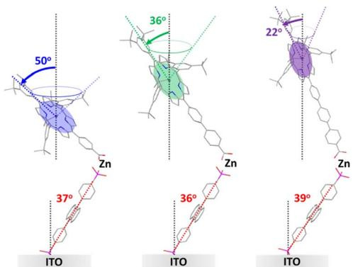
Fig. 6 Schematic representation of the mean polar tilt angles for A and PX in A-Zn-P1 (left), A-Zn-P2 (middle), and A-Zn-P3 (right) on ITO. Cones represent possible porphyrin orientations assuming the plane of the porphyrin is aligned with the axis of the phenylene carboxylate linker.
