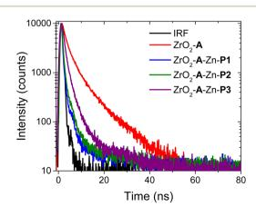
Fig. 3 Time-resolved emission at 460 nm for ZrO<sub>2</sub>-A and ZrO<sub>2</sub>-A-Zn-**PX** in MeCN ( $\lambda_{ex} = 360 \text{ nm}$ ).
