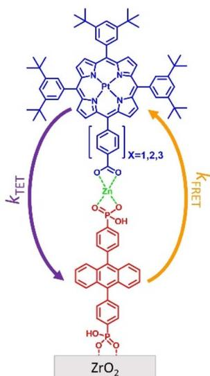
Fig. 1 General depiction of a metal ion linked bilayer composed of a  $\text{ZrO}_2$  substrate, **A** (red), Zn(II) linking ion (green), and **PX** (blue) where  $X$  is the number of phenylene spacers. The directionality and rate constant for TET and FRET are depicted in purple and orange, respectively.
