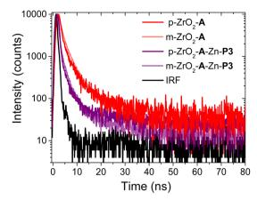
Fig. 5 Time-resolved emission decays at 460 nm for planar (p-) and mesoporous (m-)  $ZrO_2$ -A and  $ZrO_2$ -A-Zn-P3 in MeCN ( $\lambda_{ex}$  = 360 nm).
