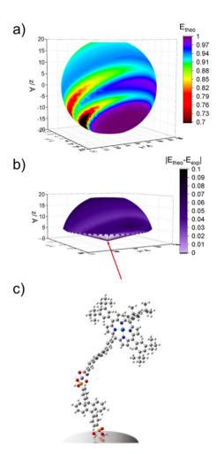
Fig. 8 (a) Calculated A to P3 FRET efficiencies for ZrO<sub>2</sub>-A-Zn-P3 where  $\theta_A$  is 39° and P3 is oriented at all geometries with a porphyrin core plane angle of 22° relative to surface normal. (b) Heatmap depicting absolute difference between theoretical and experimental FRET efficiencies. (c) Example geometry of a bilayer orientation within the feasible band ( $\theta_P = 53^\circ$ ,  $\varphi = 21^\circ$ ,  $\theta_{rot} = 62^\circ$ ).
