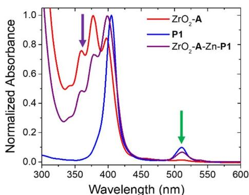
Fig. 2 Absorption spectra of ZrO<sub>2</sub>-**A**, ZrO<sub>2</sub>-**A**-Zn-**P1**, and **P1** in chloroform:methanol (1 : 1, v/v). Purple and green arrows indicate 360 and 512 nm excitation wavelengths, respectively.
