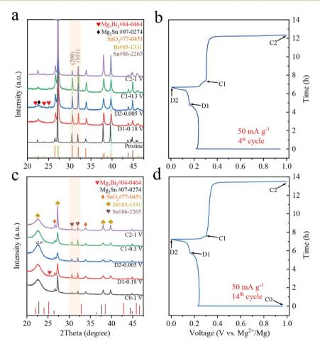
Fig. 6 The ex situ XRD patterns and corresponding the discharge/charge curves of the BSS-600 electrodes in the varied states of the 4<sup>th</sup> cycle (a and b) and the 14th cycle (c and d).
