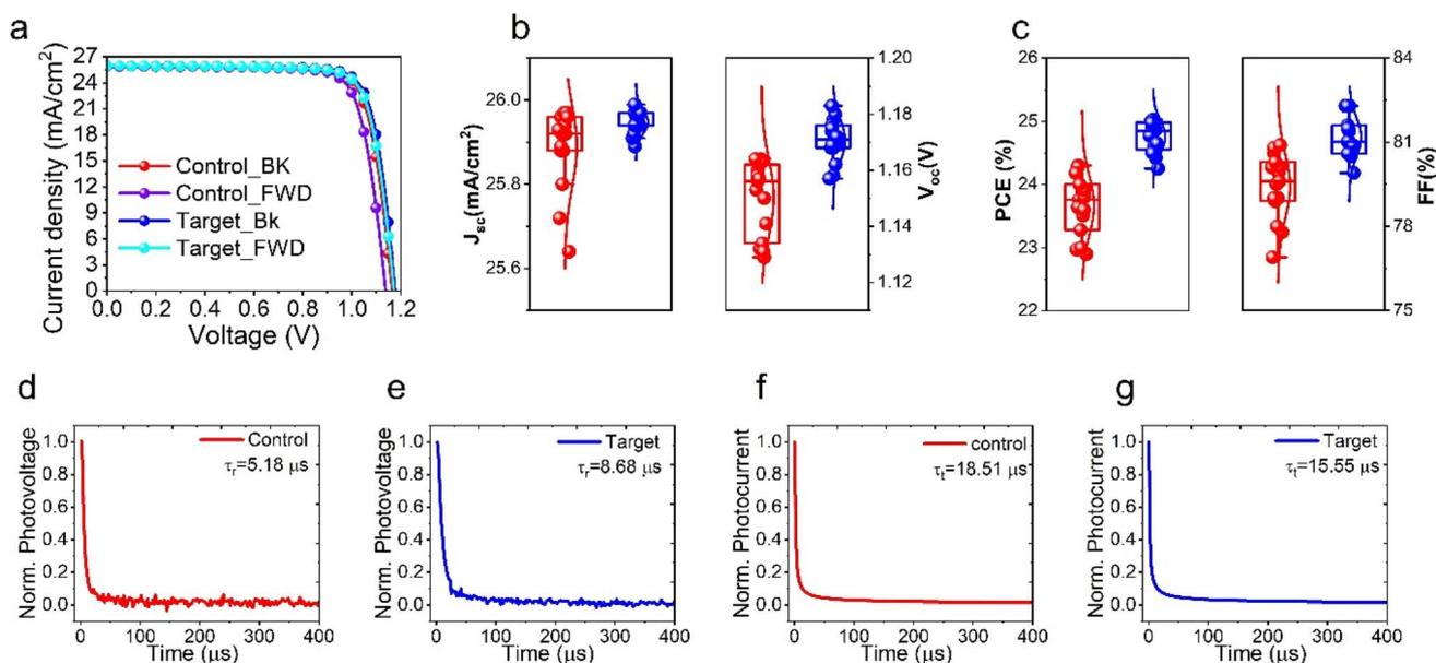
Fig. 2 Optoelectronic properties: (a)  $J$ - $V$  curves of the champion control and target solar cells under reverse and forward scans. (b and c) Summary of photovoltaic metrics ( $V_{oc}$ ,  $J_{sc}$ , PCE, and FF) of the devices (red: control; blue: target). (d and e) Normalized transient photovoltage of control and target devices, respectively. (f and g) Normalized transient photocurrent of control and target devices, respectively.
