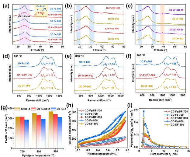
**Fig. 2** (a) The XRD patterns of the 3D Fe/DF-X and 3D Fe-X catalysts; (b) 3D DF-X supports and 3D Fe/DF-X catalysts; (c) 3D DF-800-R and 3D DF-900-R; (d–f) Raman spectra of the 3D DF-X support, 3D Fe/DF-X, and 3D Fe-X catalysts; (g) the full width at half maximum of the carbon D band for all samples; (h)  $N_2$  sorption isotherms and (i) pore size distributions of 3D Fe/DF-700, 3D Fe-700, 3D Fe/DF-800, 3D Fe-800, and 3D DF-800.
