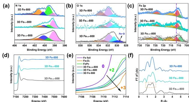
Fig. 7 Deconvoluted (a) N 1s, (b) O 1s, and (c) Fe 2p XPS spectra of 3D Fe<sub>0.25</sub>-800, 3D Fe<sub>0.5</sub>-800, and 3D Fe-800; Fe K-edge (d and e) XANES spectra and (f) FT-EXAFS spectra of 3D Fe<sub>0.25</sub>-800, 3D Fe<sub>0.5</sub>-800, and 3D Fe-800.
