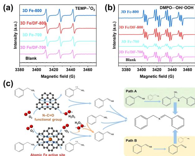
Fig. 10 EPR signals of (a) TEMP- $^1\text{O}_2$  adduct, and (b) DMPO- $\cdot\text{OH}/\cdot\text{OOH}$  adducts in the presence of 3D Fe/DF-700, 3D Fe-700, 3D Fe/DF-800, and 3D Fe-800 at 110 °C; (c) proposed reaction mechanism for the oxidative coupling of benzylamine.
