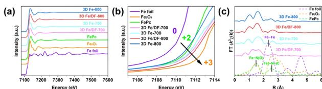
Fig. 6 Fe K-edge (a and b) XANES spectra and (c) FT-EXAFS spectra of 3D Fe/DF-700, 3D Fe-700, 3D Fe/DF-800, and 3D Fe-800, with Fe foil, Fe<sub>2</sub>O<sub>3</sub>, and FePc as reference samples.
