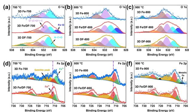
Fig. 5 (a–c) Deconvoluted O 1s XP spectra of the 3D Fe/DF-*X* and 3D Fe-*X* series with the comparison of the 3D DF-*X* supports; (d–f) deconvoluted Fe 2p XP spectra of the 3D Fe/DF-*X* and 3D Fe-*X* series.
