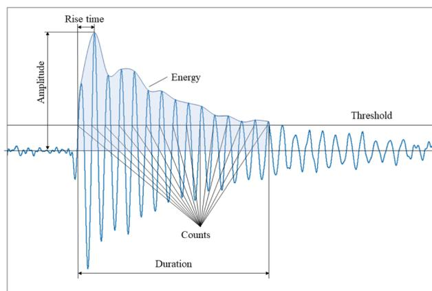
Fig. 2 Features of typical AE waveform.
