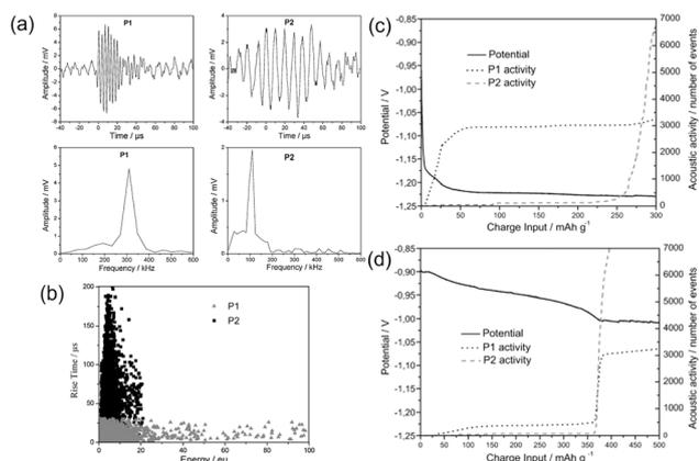
Fig. 4 (a) Typical waveforms and (b) waveform distributions of P1- and P2-type events. Electrode potential and acoustic activity as functions of time for (c) LaNi<sub>5</sub>-based and (d) MgNi electrodes. Reproduced with permission from ref. 45. Copyright 2011, Elsevier.
