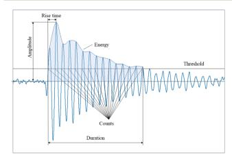
Fig. 2 Features of typical AE waveform.
