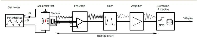
Fig. 1 The sensor chain for detecting and analyzing acoustic emissions from battery cells in research and development.
