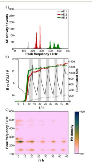
Fig. 8 (a) Distribution of peak frequencies of an HEO electrode. (b) Voltage profile and corresponding cumulated hits for different peak frequency ranges. (c) Contour plot of peak frequency as a function of time. Reproduced with permission from ref. 32. Copyright 2021, Nature Portfolio.
