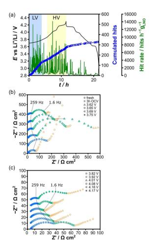
Fig. 9 (a) Voltage profile of the initial cycle of an LNO half-cell. (b) Low-voltage and (c) high-voltage regions Nyquist plots of the EIS data. Reproduced with permission from ref. 19. Copyright 2020, Wiley-VCH.
