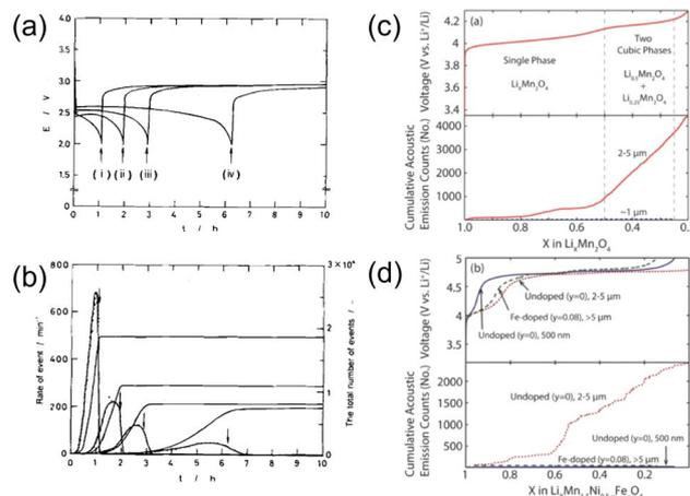
Fig. 10 (a) Discharge profiles and (b) corresponding AE hit rates of MnO<sub>2</sub>. Reproduced with permission from ref. 40. Copyright 1997, The Electrochemical Society. Voltage profiles and cumulative AE hits of (c) LiMn<sub>2</sub>O<sub>4</sub> and (d) LiMn<sub>1.5</sub>Ni<sub>0.5</sub>O<sub>4</sub>. Reproduced with permission from ref. 60. Copyright 2014, The Electrochemical Society.
