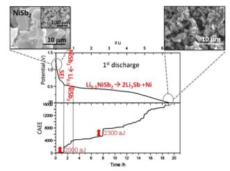
Fig. 7 Voltage profile and cumulated AE energy of NiSb<sub>2</sub>/Li cell as functions of time. Reproduced with permission from ref. 31. Copyright 2010, Elsevier.
