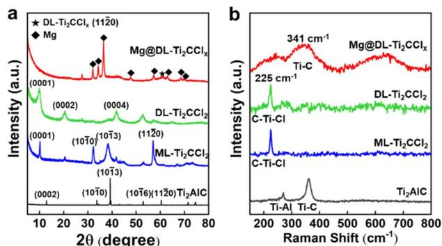
Fig. 2 Change of the crystalline and chemical structures of the  $\text{Ti}_2\text{AlC}$  MAX phase,  $\text{ML-Ti}_2\text{CCl}_2$ ,  $\text{DL-Ti}_2\text{CCl}_2$  and  $\text{Mg@DL-Ti}_2\text{CCl}_2$  composite based on (a) X-ray diffraction (XRD) patterns and (b) Raman spectra.
