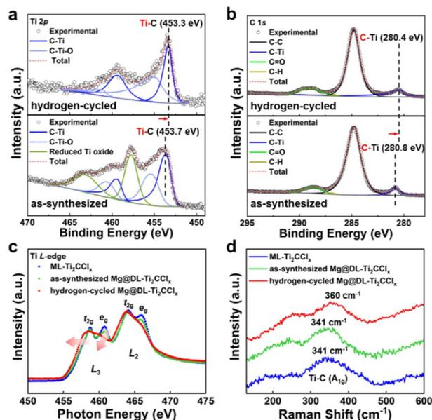
Fig. 4 Charge transfer between  $\text{DL-Ti}_2\text{CCl}_x$  and Mg. (a) Ti 2p and (b) C 1s XPS spectra of as-synthesized  $\text{Mg@DL-Ti}_2\text{CCl}_x$  (below) and hydrogen-cycled  $\text{Mg@DL-Ti}_2\text{CCl}_x$  (upper). (c) Ti L-edge NEXAFS and (d) Raman spectra of  $\text{ML-Ti}_2\text{CCl}_x$ , as-synthesized and hydrogen-cycled  $\text{Mg@DL-Ti}_2\text{CCl}_x$ .
