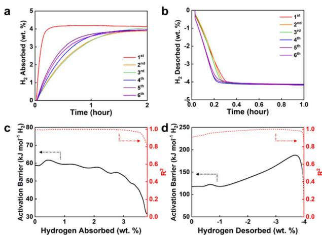
Fig. 3 Hydrogen sorption kinetics of the  $\text{Mg@DL-Ti}_2\text{CCl}_2$  composite. (a) Isothermal hydrogen absorption at 200 °C under 15 bar of  $\text{H}_2$  and (b) hydrogen desorption at 300 °C under 0 bar of  $\text{H}_2$ . Activation barrier for (c) absorption and (d) desorption as a function of absorbed and desorbed wt%  $\text{H}_2$ , respectively.
