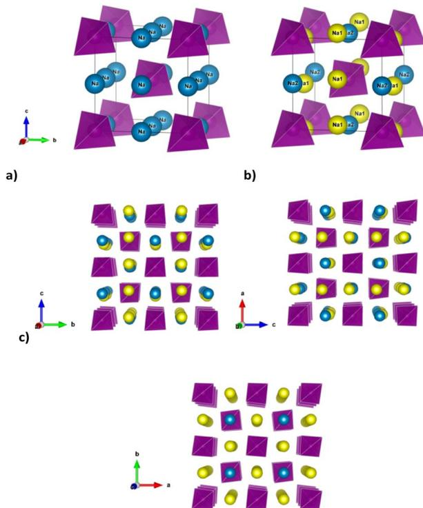
Fig. 1 Cubic (a) and tetragonal structure (b) of  $\text{Na}_{3-x}\text{Sb}_{1-x}\text{W}_x\text{S}_4$  showing the presence of two Na crystallographic sites for the tetragonal polymorph due to the lower symmetry. Panel (c) shows three perspective views along the three crystallographic axes for the tetragonal polymorph, to highlight the presence of distinct diffusion channels for Na ions, involving Na1 and Na2 along the *a* and *b* axes and only Na1 along the *c* axis.
