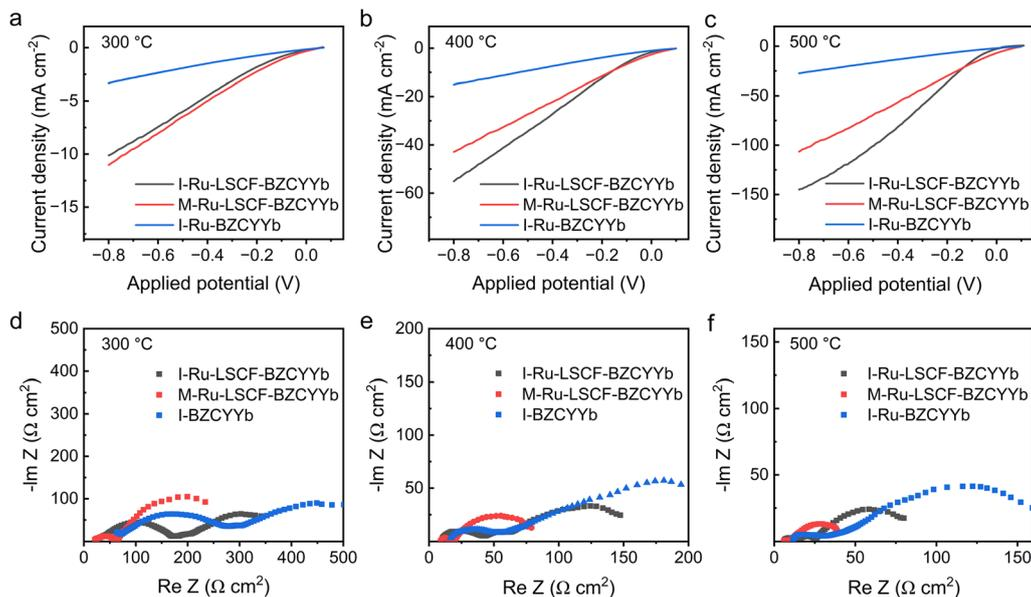
Fig. 4 (a–c)  $j$ - $E$  curves with a scan rate of  $10 \text{ mV s}^{-1}$ , and (d–f) EIS at OCV of the I-Ru-LSCF-BZCYYb|BZCYYb|Ni-BZCYYb, M-Ru-LSCF-BZCYYb|BZCYYb|Ni-BZCYYb, and I-Ru-BZCYYb|BZCYYb|Ni-BZCYYb electrolysis cells at different temperatures. Reaction gas: pure  $\text{N}_2$  at the working electrode; 5%  $\text{H}_2$ -95% Ar at the counter electrode (reference electrode).
