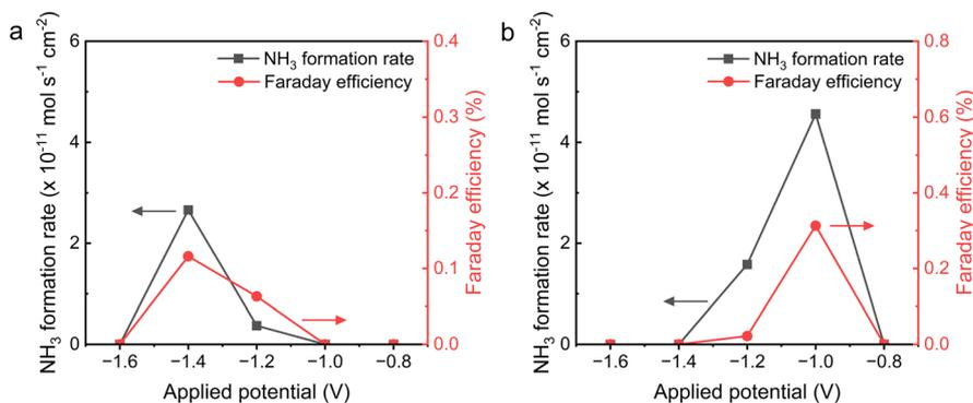
Fig. 7  $\text{NH}_3$  formation rate and Faraday efficiency of the I-Ru-LSCF-BZCYYb|BZCYYb|Ni-BZCYYb electrolysis cell at (a) 400 °C and (b) 500 °C. Reaction gas: pure  $\text{N}_2$  at the working electrode; wet Ar at the counter electrode (reference electrode).
