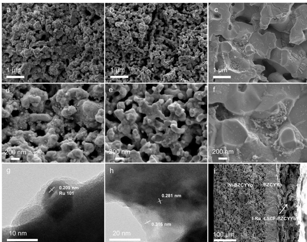
**Fig. 3** SEM images of (a and d) the I-Ru-LSCF-BZCYyb cathode, (b and e) the M-Ru-LSCF-BZCYyb cathode, and (c and f) the I-Ru-BZCYyb cathode. (g and h) HR-TEM images of the I-Ru-LSCF-BZCYyb cathode. (i) SEM image of the cross-section of the I-Ru-LSCF-BZCYyb|BZCYyb|Ni-BZCYyb electrolysis cell.
