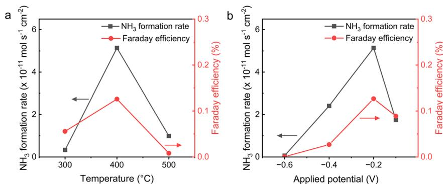
Fig. 5 NH $_3$  formation rate and Faraday efficiency of the I-Ru-LSCF-BZCYYb|BZCYYb|Ni-BZCYYb electrolysis cell (a) at different temperatures and an applied potential of  $-0.2$  V, and (b) at 400 °C and different potentials. Reaction gas: pure N $_2$  at the working electrode; 5% H $_2$ –95% Ar at the counter electrode (reference electrode).
