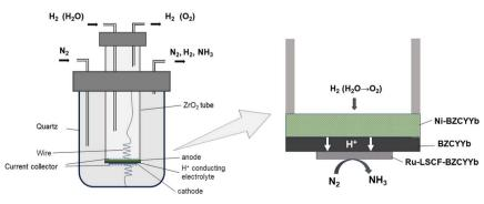
Fig. 1 Schematic diagram of a device for a PCEAS electrolysis cell.
