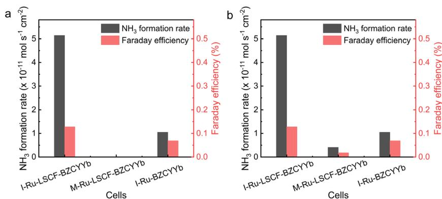
Fig. 6 Comparison of NH<sub>3</sub> formation rate and Faraday efficiency of the I-Ru-LSCF-BZCYyb|BZCYyb|Ni-BZCYyb, the M-Ru-LSCF-BZCYyb|BZCYyb|Ni-BZCYyb, and the I-Ru-BZCYyb|BZCYyb|Ni-BZCYyb electrolysis cells (a) at 400 °C and -0.2 V, and (b) under the optimum conditions. Reaction gas: pure N<sub>2</sub> at the working electrode; 5% H<sub>2</sub>-95% Ar at the counter electrode (reference electrode).
