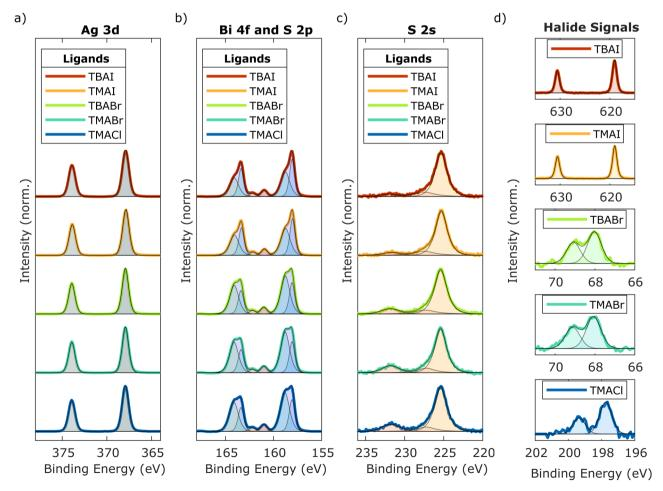
Fig. 2 XPS core level spectra of AgBiS<sub>2</sub> thin films treated with different ligands: (a) Ag 3d signal, fitted with one component, (b) overlapping Bi 4f and S 2p signals, fitted with 2 components for the Bi 4f (blue/green areas) and 1 component for the S 2p signals (red/orange areas), (c) S 2s signal, fitted with 3 components and (d) the different halide signals (I 3d, Br 3d, Cl 2p), fitted with one component each.
