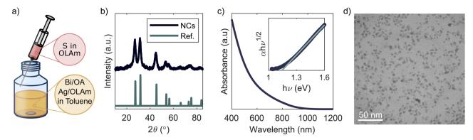
Fig. 1 AgBiS $_2$  synthesis and material characterisation: (a) synthesis scheme, (b) XRD data and ref. 24, (c) absorbance spectra with Tauc plot as inset and (d) TEM image of as-synthesised NCs.
