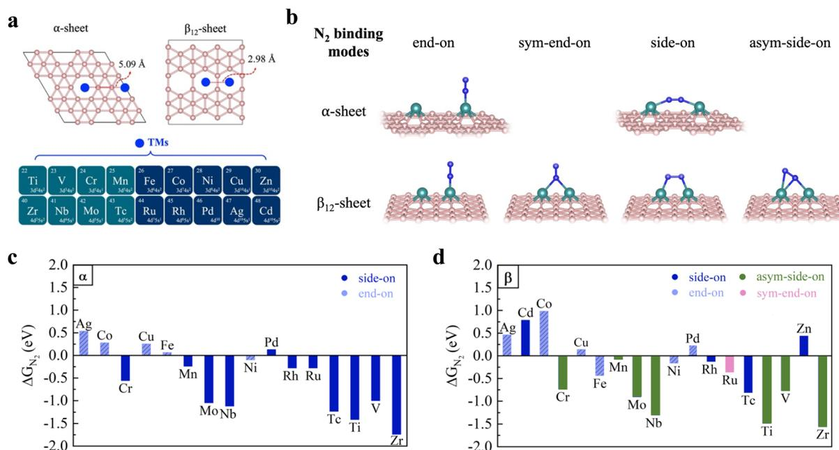
Fig. 1 (a) Dual-atom catalyst models based on boron  $\alpha$ - and  $\beta_{12}$ -sheets, and a range of transition metals used for catalyst screening. (b) Various possible N<sub>2</sub> binding configurations on DACs based on  $\alpha$ - and  $\beta_{12}$ -sheets. The most stable N<sub>2</sub> adsorption structures and energies for (c)  $\alpha$ -sheets and (d)  $\beta_{12}$ -sheets.
