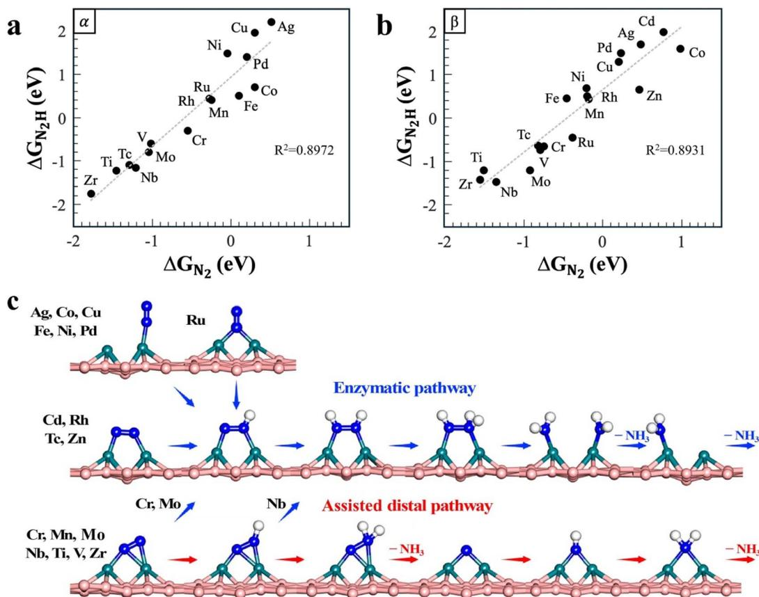
Fig. 4 Correlation between  $N_2$  and  $N_2H$  binding free energies for (a)  $\alpha$ -sheets (denoted as  $\alpha$ ) and (b)  $\beta_{12}$ -sheets (denoted as  $\beta$ ). (c) Selected eNRR pathways depending on the  $N_2$  binding structures.
