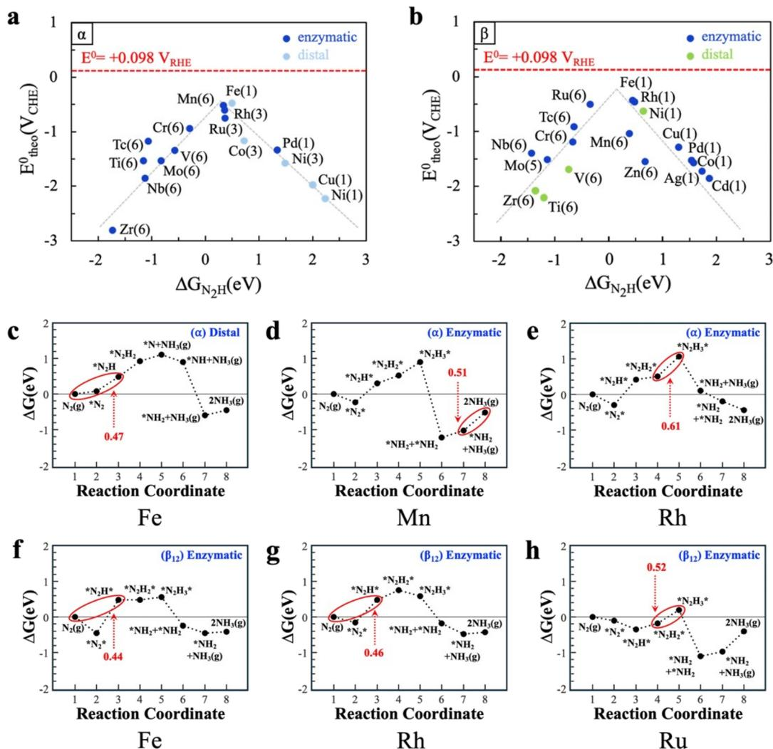
Fig. 5 Volcano plot of eNRR limiting potentials for (a)  $\alpha$ -sheets (denoted as  $\alpha$ ) and (b)  $\beta_{12}$ -sheets (denoted as  $\beta$ ). Reaction free energy profiles for (c) Fe, (d) Mn, and (e) Rh on  $\alpha$ -sheets, and for (f) Fe, (g) Rh, and (h) Ru on  $\beta_{12}$ -sheets. The potential-determining step (PDS) for each catalyst is indicated by the number in the parenthesis in graphs (a) and (b).
