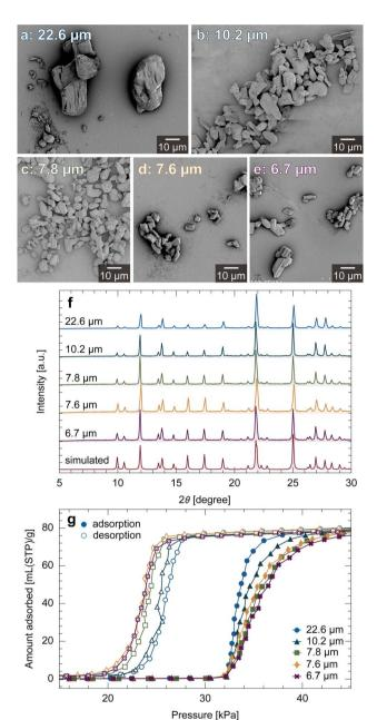
Fig. 2 (a)-(e) SEM images, (f) XRD patterns, and (g) CO<sub>2</sub> adsorption isotherms (273 K) of ELM-11 particles synthesized under various concentration conditions. The closed and open symbols in (g) represent adsorption and desorption branches, respectively.
