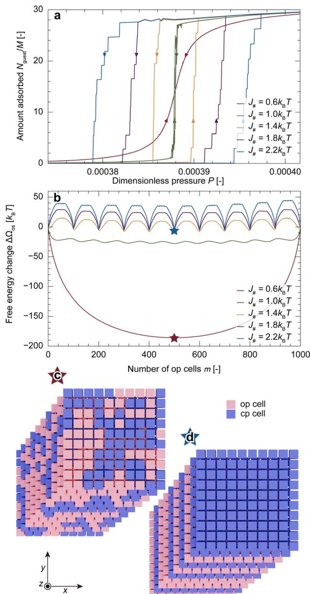
Fig. 4 (a) Adsorption isotherms for the particle model and (b) free energy profiles with various  $J_{\#}$ . (c) and (d) Display snapshots of the particle model at the points marked with star symbols in (b), where pink and blue cubes represent op and cp cells, respectively. The layers are displayed with a slight offset.
