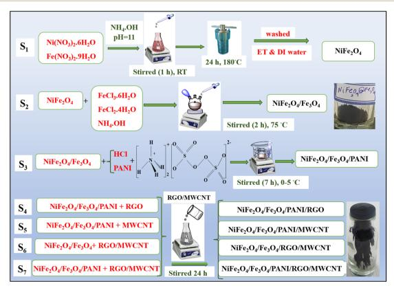
Fig. 1 Schematic representation of the synthesis of samples S<sub>1</sub>, S<sub>2</sub>, S<sub>3</sub>, S<sub>4</sub>, S<sub>5</sub>, S<sub>6</sub>, and S<sub>7</sub> at room temperature (RT).
