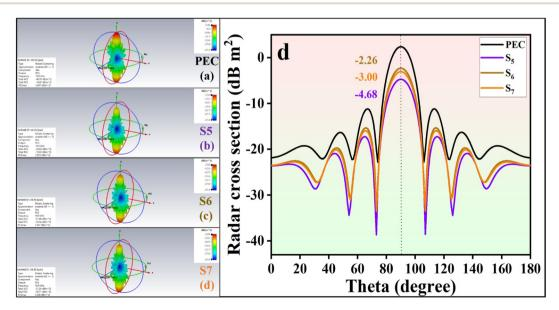
Fig. 20 3D intensity images of the reflected signal PEC (a), PEC coated with S<sub>5</sub>, S<sub>6</sub>, S<sub>7</sub>, and RCS simulated curves of the samples at different scanning angles (d).
