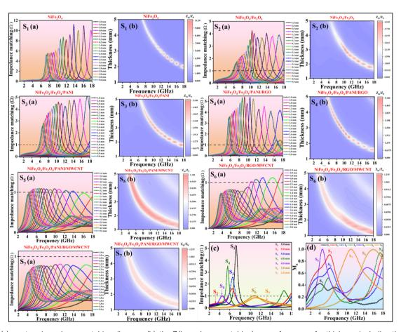
Fig. 13 2D (a), contour impedance matching diagrams (b), the Z (impedance matching) versus frequency for thickness including the best RL<sub>min</sub> (c), the best input impedance matching coefficient ( $M_z$ ) (d) of S<sub>1</sub>, S<sub>2</sub>, S<sub>3</sub>, S<sub>4</sub>, S<sub>5</sub>, S<sub>6</sub>, S<sub>7</sub>.
