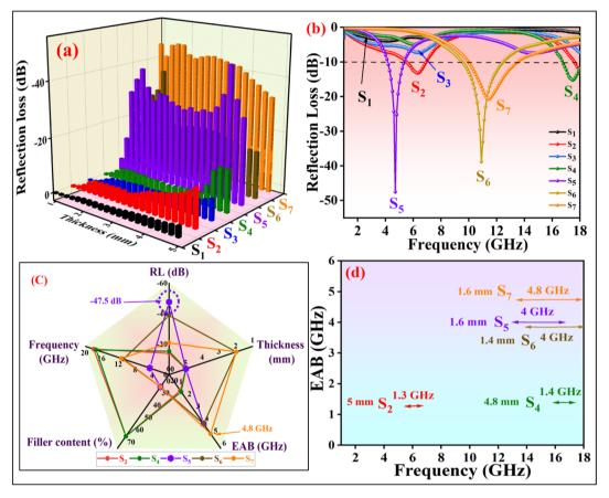
Fig. 11 (a) Reflection loss of all samples, (b) the best RL<sub>min</sub>, (c) radar chart, (d) EAB for: (S<sub>1</sub>) NiFe<sub>2</sub>O<sub>4</sub>, (S<sub>2</sub>) NiFe<sub>2</sub>O<sub>4</sub>/Fe<sub>3</sub>O<sub>4</sub>, (S<sub>3</sub>) NiFe<sub>2</sub>O<sub>4</sub>/Fe<sub>3</sub>O<sub>4</sub>/PANI,  $(S_4)\ NiFe_2O_4/Fe_3O_4/PANI/RGO, (S_5)\ NiFe_2O_4/Fe_3O_4/PANI/MWCNT, (S_6)\ NiFe_2O_4/Fe_3O_4/RGO/MWCNT, (S_7)\ NiFe_2O_4/Fe_3O_4/PANI/RGO/MWCNT.$
