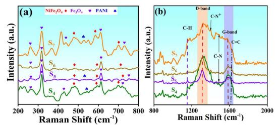
Fig. 3 Raman spectrum obtained for  $S_4$ ,  $S_5$ ,  $S_6$ , and  $S_7$  in different ranges from (a):  $(200-800 \text{ cm}^{-1})$  and (b):  $(800-2000 \text{ cm}^{-1})$ .
