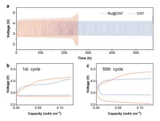
Fig. 5 (a) Cycle performance of LOBs with CNTs or Ru@CNT additive (CNT content: 1.0 mg mL<sup>-1</sup>, current density: 0.05 mA cm<sup>-2</sup>, and areal capacity: 0.125 mA h cm<sup>-2</sup>). The discharge and charge curves of the (b) 1st cycle and (c) 55th cycle.
