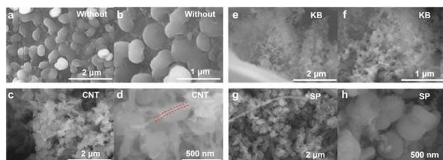
Fig. 1 Scanning electron microscope (SEM) images of the cathodes discharged to 2 V at  $0.1 \text{ mA cm}^{-2}$ . (a and b) Without a conductive additive. (c and d) With  $3 \text{ mg mL}^{-1}$  CNTs. (e and f) With  $3 \text{ mg mL}^{-1}$  KB. (g and h) With  $3 \text{ mg mL}^{-1}$  SP.
