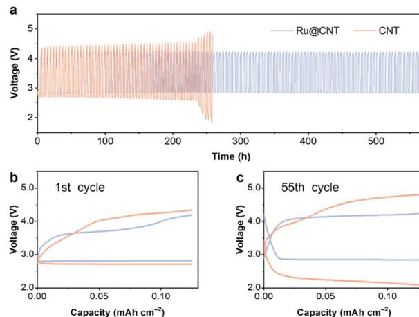
Fig. 5 (a) Cycle performance of LOBs with CNTs or Ru@CNT additive (CNT content:  $1.0 \text{ mg mL}^{-1}$ , current density:  $0.05 \text{ mA cm}^{-2}$ , and areal capacity:  $0.125 \text{ mA h cm}^{-2}$ ). The discharge and charge curves of the (b) 1st cycle and (c) 55th cycle.
