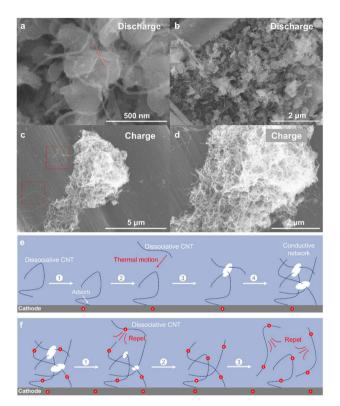
Fig. 4 SEM images of the cathodes of LOBs with 1.0 mg mL<sup>-1</sup> CNTs after the first (a and b) discharge and (c and d) charge processes. A schematic illustration of the function of CNTs in the (e) discharge and (f) charge processes
