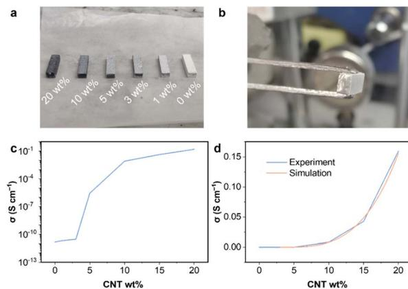
Fig. 3 (a) Optical images of  $\text{Li}_2\text{O}_2$  samples mixed with different amounts of CNTs. (b) The end face of a sample that is covered with silver paste. (c) Relationship between the conductivity and the CNT content. (d) Comparison curves of the experimental and calculated conductivities.
