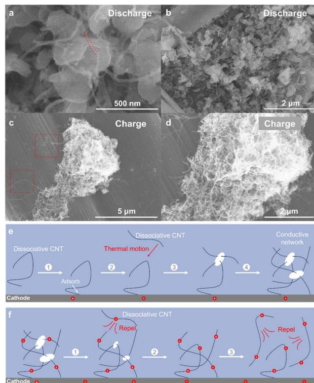
Fig. 4 SEM images of the cathodes of LOBs with  $1.0 \text{ mg mL}^{-1}$  CNTs after the first (a and b) discharge and (c and d) charge processes. A schematic illustration of the function of CNTs in the (e) discharge and (f) charge processes.
