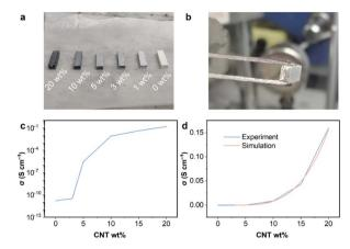
Fig. 3 (a) Optical images of Li<sub>2</sub>O<sub>2</sub> samples mixed with different amounts of CNTs. (b) The end face of a sample that is covered with silver paste. (c) Relationship between the conductivity and the CNT content. (d) Comparison curves of the experimental and calculated conductivities
