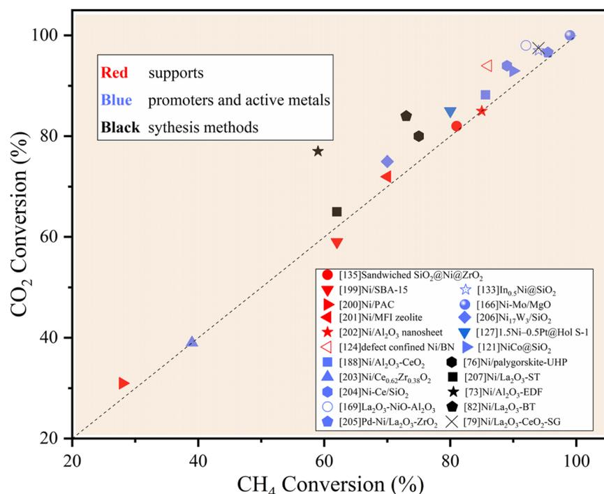
Fig. 21 The comparison diagram of CH<sub>4</sub> and CO<sub>2</sub> conversion of different catalysts at 800 °C.
