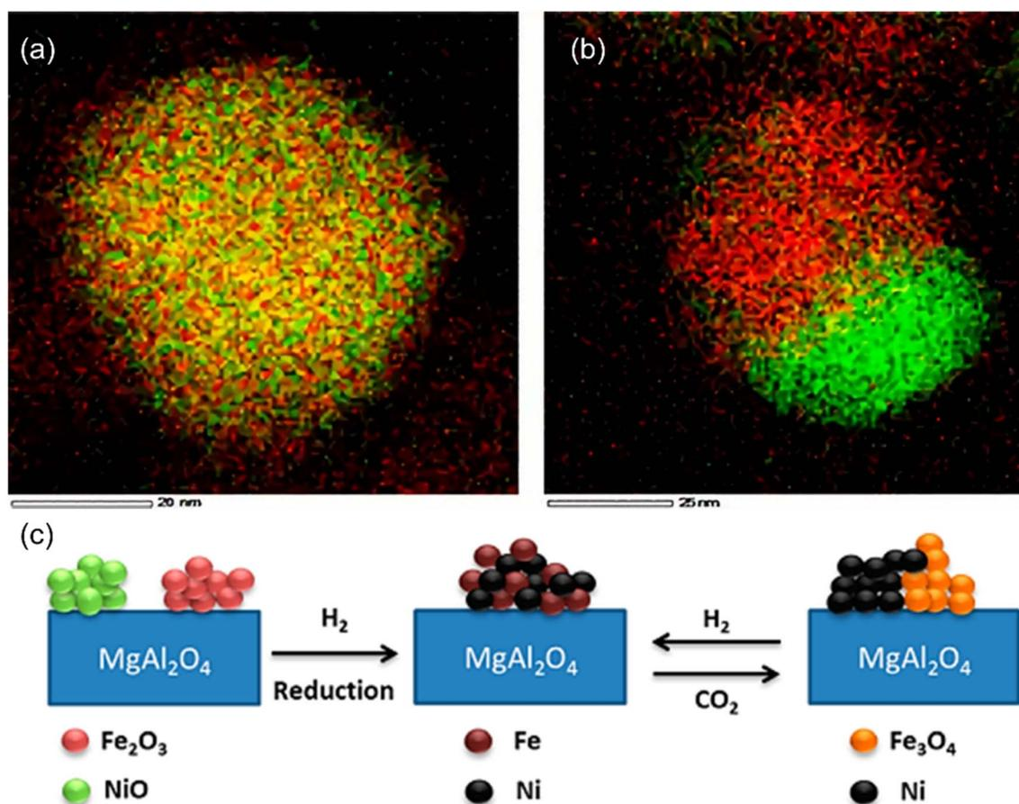
Fig. 17 EDX element mapping of 0.7-Fe/Ni (a) after H<sub>2</sub> reduction and (b) after CO<sub>2</sub> oxidation during DRM reaction. (c) Schematic diagram of the effect of Fe–Ni alloy on CO<sub>2</sub> activation and coke elimination. Reprinted with permission from ref. 180 Copyright 2015, American Chemical Society.
