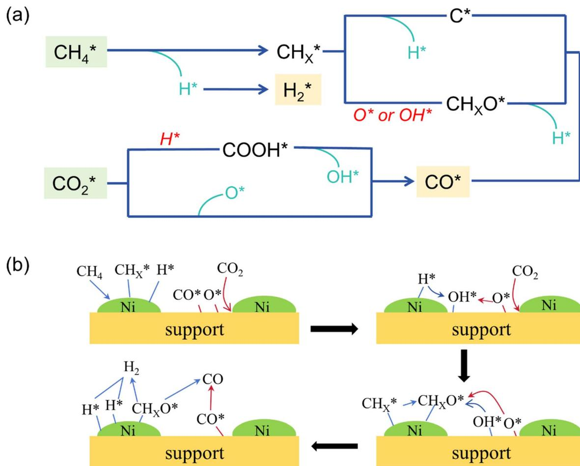
Fig. 5 (a) Principal steps of DRM reaction. (b) Active sites and molecular conversion on the catalyst surface in DRM reaction, which shows the dissociation of  $\text{CH}_4$  and  $\text{CO}_2$ , formation of  $\text{OH}^*$  and  $\text{CH}_x\text{O}^*$ , decomposition of  $\text{CH}_x\text{O}^*$ , and release of  $\text{CO}$  and  $\text{H}_2$ .
