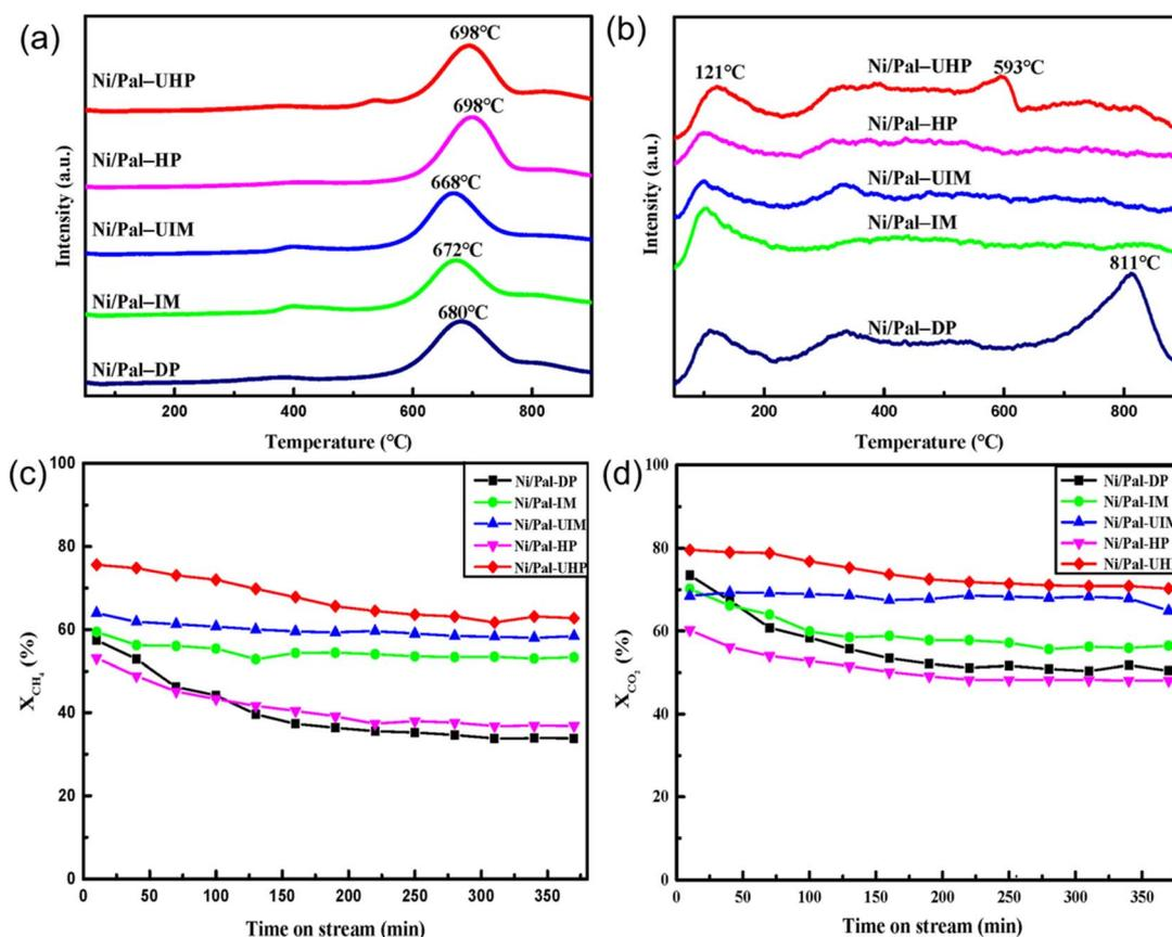
Fig. 8 (a) H<sub>2</sub>-TPR profiles, (b) CO<sub>2</sub>-TPD profiles, (c) CH<sub>4</sub> conversion, and (d) CO<sub>2</sub> conversion for Ni/Pal with different preparation methods. Reprinted with permission from ref. 92 Copyright 2022, Elsevier.
