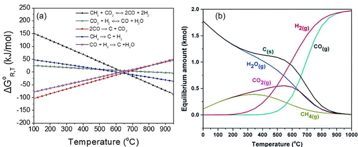
Fig. 2 Thermodynamic analysis at equilibrium calculated as a function of temperature. (a)  $\Delta G_{R,T}^{\circ}$  of all the reactions involved in the DRM process at 1 bar. Reprinted with permission from ref. 16 Copyright 2021, Elsevier. (b) Equilibrium data of chemical compounds for DRM. Reprinted with permission from ref. 29 Copyright 2016, The Royal Society of Chemistry.
