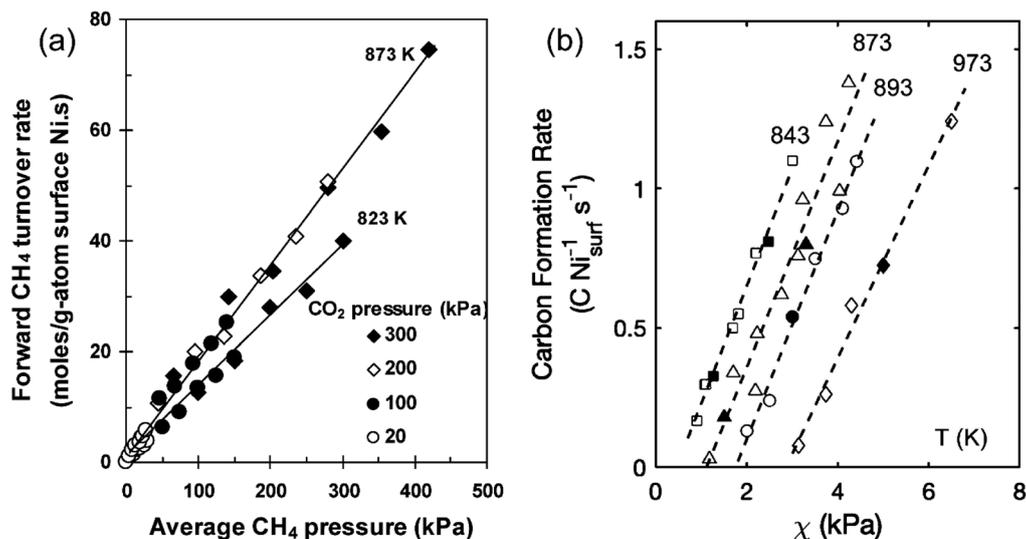
Fig. 3 The kinetic mechanism of reactant decomposition and carbon deposition in reforming reactions. (a) Effects of CH<sub>4</sub> pressure on forward CH<sub>4</sub> reaction rate for DRM on Ni/MgO. Reprinted with permission from ref. 30 Copyright 2004, Elsevier. (b)  $\chi$  ( $P_{\text{CH}_4}P_{\text{CO}}/P_{\text{CO}_2}$ ) on carbon formation rates for DRM on Ni/MgO (open symbol). Reprinted with permission from ref. 31 Copyright 2020, American Chemical Society.
