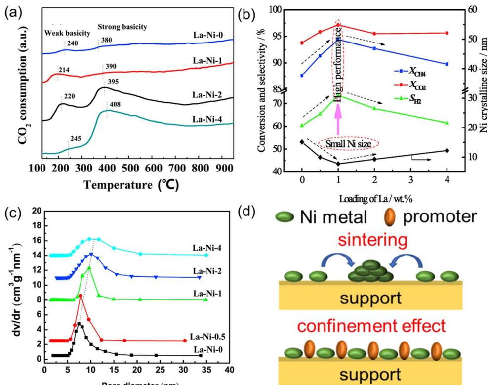
Fig. 18 The effect of La<sub>2</sub>O<sub>3</sub> promoters. (a) CO<sub>2</sub>-TPD profiles with different La loading. (b) The catalytic performance and Ni crystalline size with different La loading (wt%). (c) Pore diameter distributions of catalysts with different La loading. Reprinted with permission from ref. 169 Copyright 2019, Elsevier. (d) Schematic diagram of the anti-sintering mechanism of promoters.
