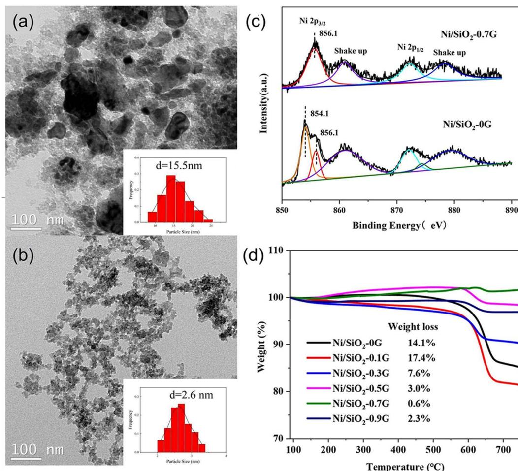
Fig. 7 TEM images of reduced catalysts of (a) Ni/ $\text{SiO}_2$ -0G and (b) Ni/ $\text{SiO}_2$ -0.7G. (c) Ni 2p X-ray photoelectron spectra of fresh catalysts. (d) TGA profiles for spent catalysts. Reprinted with permission from ref. 73 Copyright 2022, Elsevier.
