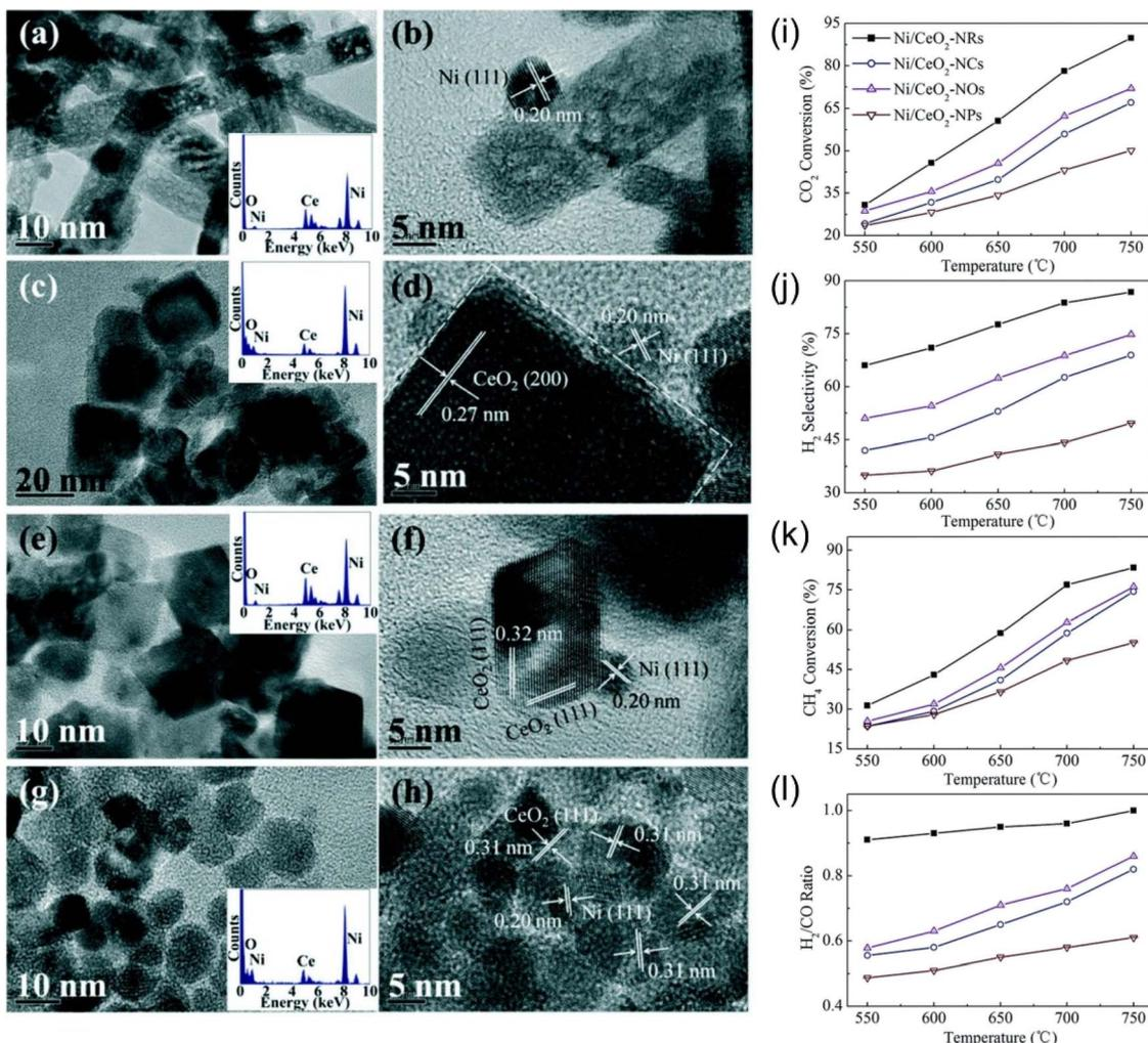
Fig. 10 TEM, HRTEM, SAED (inset) images of CeO<sub>2</sub>: (a and b) rods, (c and d) cubes, (e and f) octahedrons, and (g and h) particles. (i–l) Catalytic performance with different CeO<sub>2</sub> morphology over different temperatures. Reprinted with permission from ref. 115 Copyright 2016, The Royal Society of Chemistry.
