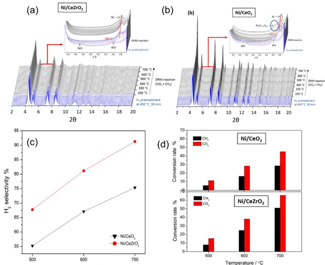
Fig. 15 *In situ* XRD profiles of (a) Ni/CeZrO<sub>2</sub> and (b) Ni/CeO<sub>2</sub> samples under different DRM reaction temperatures. (c) The H<sub>2</sub> selectivity and (d) reactants conversion for the DRM reaction over Ni/CeO<sub>2</sub> and Ni/CeZrO<sub>2</sub> samples. Reprinted with permission from ref. 157 Copyright 2020, American Chemical Society.
