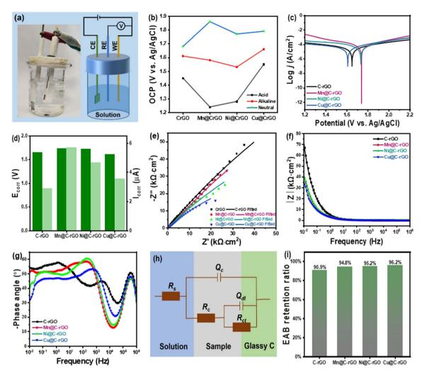
Fig. 9 (a) Schematic of the three-electrode system. (b) The OCP values under acidic, neutral, and alkaline environments. (c) The Tafel curves and (d) the  $E_{corr}$  and  $I_{corr}$  under neutral corrosion conditions. (e) The Nyquist plots, (f) Bode plots and (q) phase angle plots of four absorbers in neutral solutions. (h) The equivalent circuit and (i) the retained ratio of EAB after soaking in 3.5 wt% NaCl solution for 7 days.
