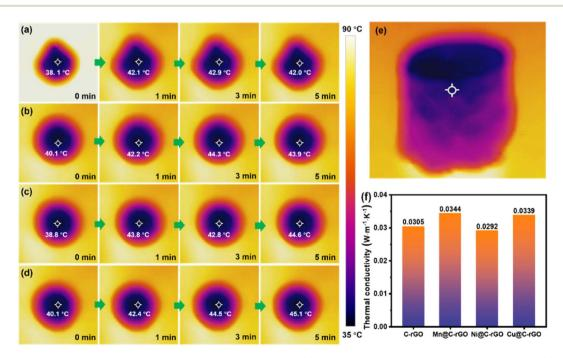
Fig. 8 The infrared images of (a) C-rGO, (b) Mn@C-rGO, (c) Ni@C-rGO and (d) Cu@C-rGO placed on the heat source at 90 °C. (e) The side-view infrared image of Cu@C-rGO and (f) thermal conductivity.
