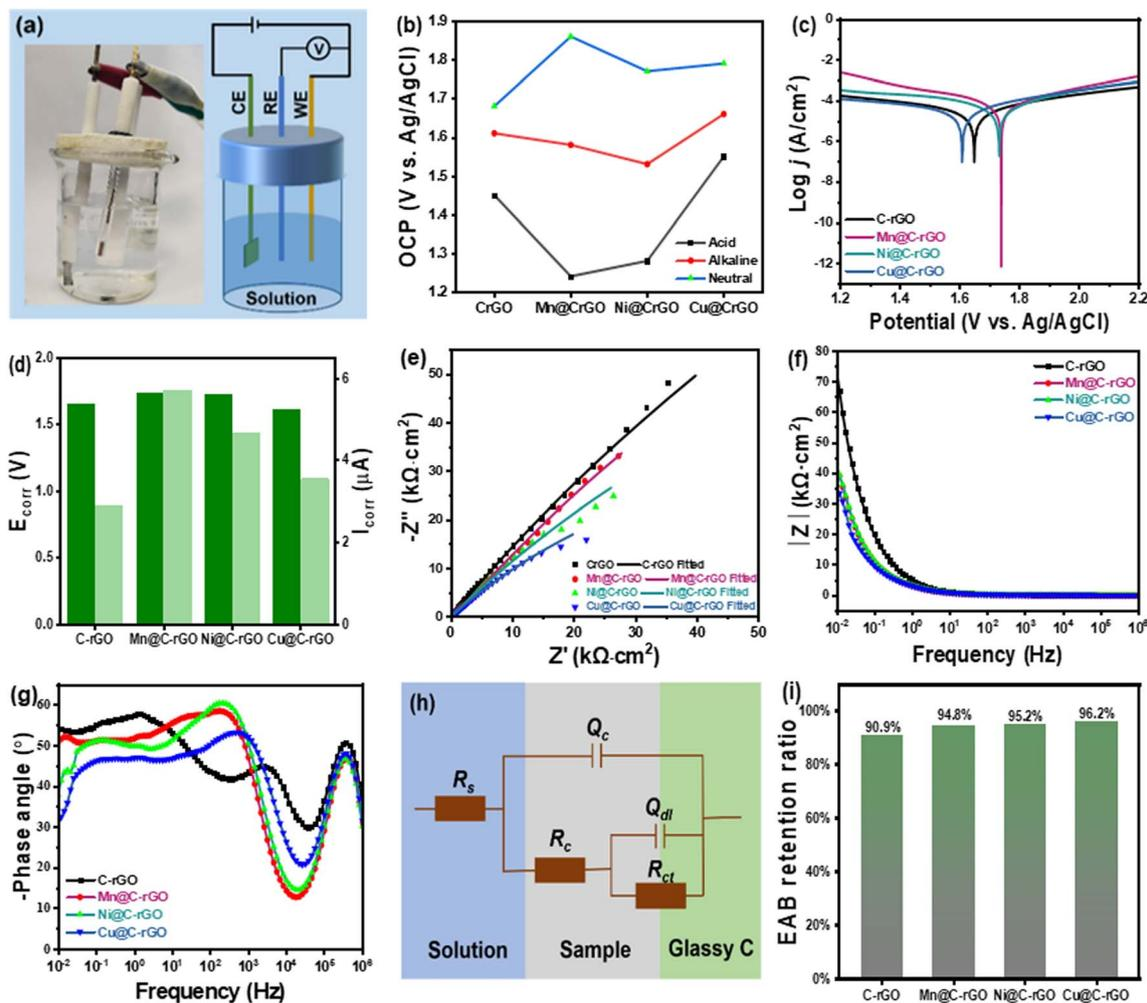
Fig. 9 (a) Schematic of the three-electrode system. (b) The OCP values under acidic, neutral, and alkaline environments. (c) The Tafel curves and (d) the  $E_{\text{corr}}$  and  $I_{\text{corr}}$  under neutral corrosion conditions. (e) The Nyquist plots, (f) Bode plots and (g) phase angle plots of four absorbers in neutral solutions. (h) The equivalent circuit and (i) the retained ratio of EAB after soaking in 3.5 wt% NaCl solution for 7 days.
