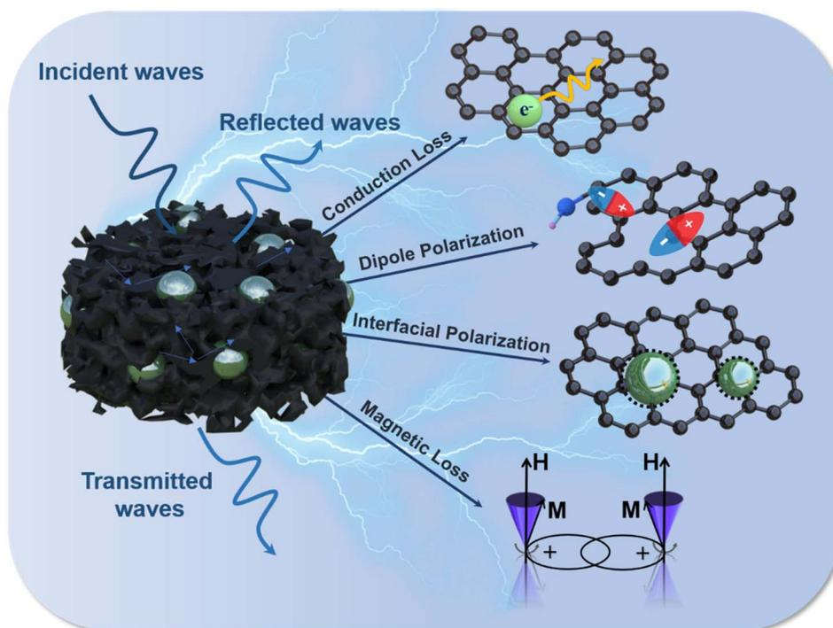
Fig. 7 Schematic illustration of microwave absorption mechanisms for the M@C-rGO.
