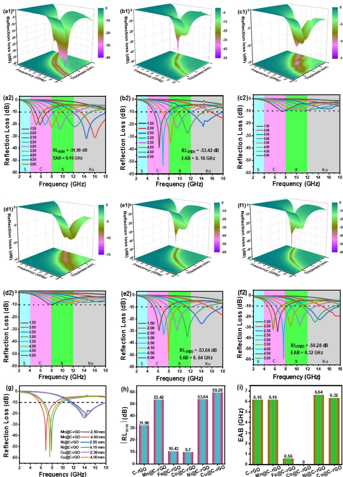
Fig. 3 The 3D RL contour plots and RL values of (a) C-rGO, (b) Mn@C-rGO, (c) Fe@C-rGO, (d) Co@C-rGO, (e) Ni@C-rGO and (f) Cu@C-rGO. The comparison of (g) RL values, (h) RL<sub>min</sub> and (i) EAB for samples.
