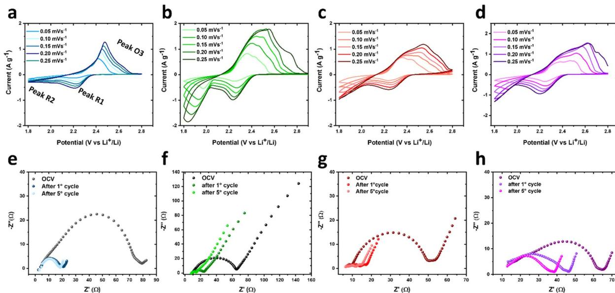
Fig. 2 (a)–(d) CV curves measured at different voltage scan rates ranging from 0.05 to 0.25  $\text{mV s}^{-1}$  for the LSBs based on (a) pristine Celgard, (b) KS60@Celgard, (c) K60@Celgard and (d) KS80@Celgard separators. (e)–(h) Nyquist plots measured for the LSBs based on (e) pristine Celgard, (f) KS60@Celgard, (g) K60@Celgard and (h) KS80@Celgard separators.
