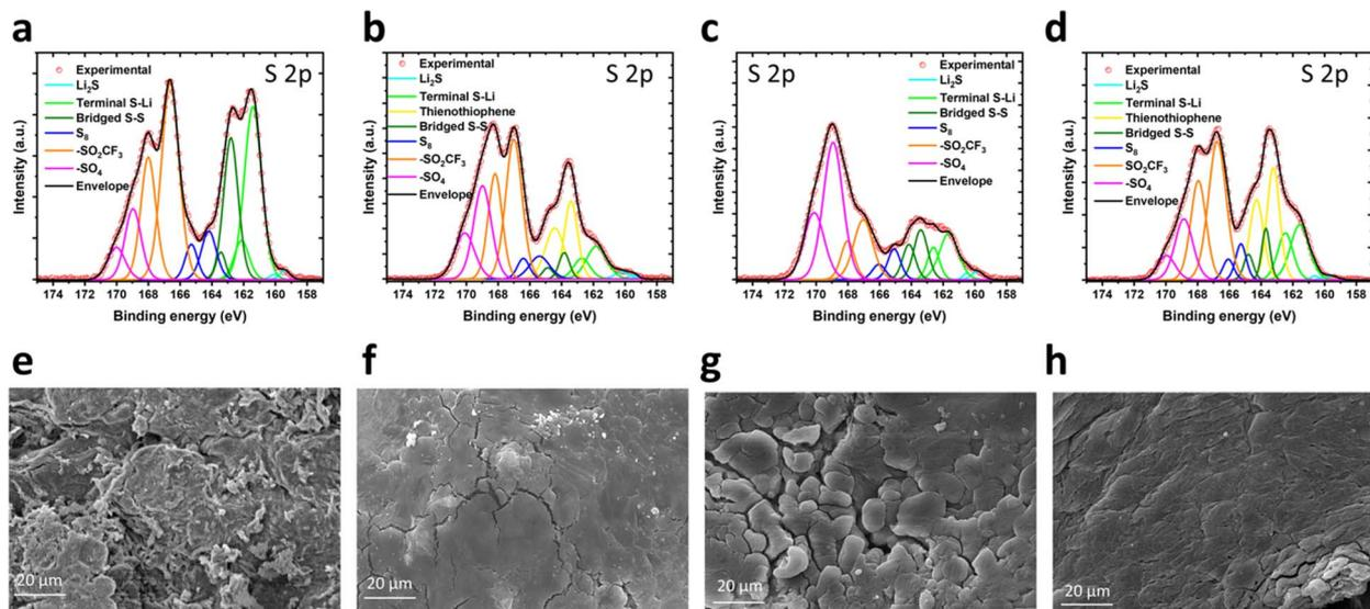
Fig. 5 *Ex situ* XPS spectra for S 2p core levels of (a) pristine Celgard, (b) KS60@Celgard, (c) K60@Celgard and (d) KS80@Celgard separators, obtained by disassembling the corresponding LSBs in the charged state after 190 GCD cycles. SEM images of Li anodes obtained by disassembling the LSBs, containing (e) pristine Celgard, (f) KS60@Celgard, (g) K60@Celgard, and (h) KS80@Celgard separators, in the charged state after 190 GCD cycles.
