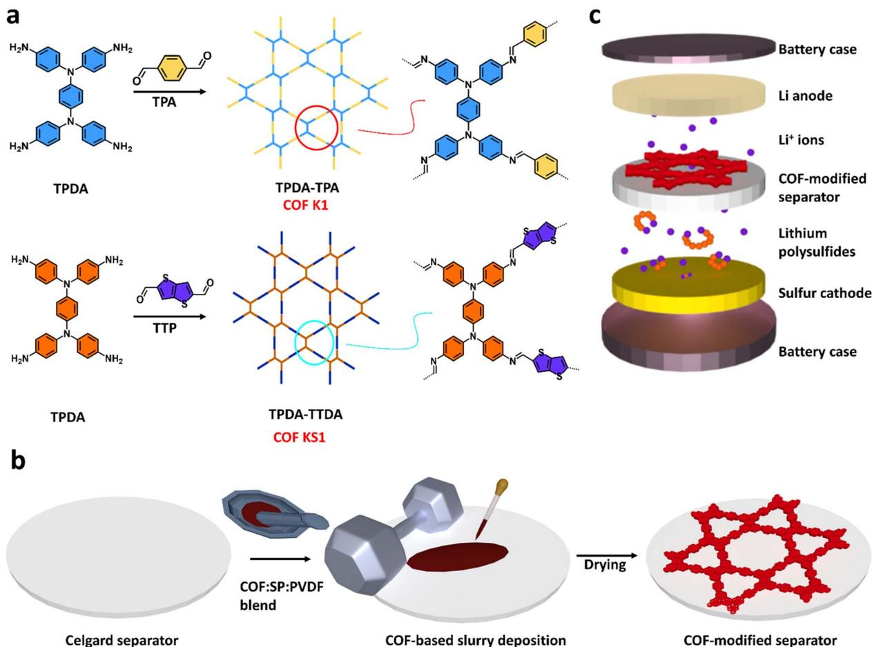
**Scheme 1** (a) Schematic representation of the solvothermal synthesis of the two Kagome shaped imine-based COFs K1 and KS1. (b) Coating of a prototypical Celgard separator with the COF : SP : PVDF blend to prepare the COF-modified separator. (c) Sketch of a LSB in coin cell format, containing a sulphur cathode, the COF-modified separator and the Li anode. The ability of the separators to block the shuttle of  $\text{Li}_2\text{S}_x$  is pictorially presented.
