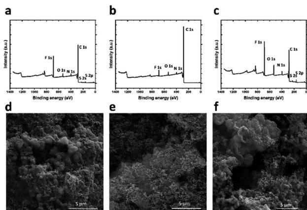
**Fig. 1** (a)–(c) Survey XPS spectra for (a) KS60@Celgard, (b) K60@Celgard and (c) KS80@Celgard separators. (d)–(f) SEM images of the (d) KS60@Celgard, (e) K60@Celgard and (f) KS80@Celgard separators.
