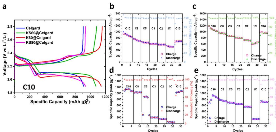
Fig. 3 (a) GCD profiles recorded at C10 of the LSBs (sulphur loading:  $\sim 2 \text{ mg}_\text{s} \text{ cm}^{-2}$ ; E/S ratio:  $15 \mu\text{L mg}_\text{s}^{-1}$ , electrode geometric area:  $1.54 \text{ cm}^2$ ) containing pristine Celgard, KS60@Celgard, K60@Celgard and KS80@Celgard separators. Rate performance from C10 to 1C of the Li–S batteries containing (b) pristine Celgard, (c) KS60@Celgard, (d) K60@Celgard and (e) KS80@Celgard separators.
