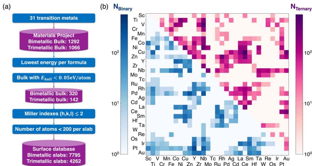
Fig. 1 High-throughput workflow and coverage of chemical space. (a) Schematic figure of the workflow for generating intermetallic surfaces. Blue boxes represent selection criteria and purple areas represent the description of the database. (b) Coverage of chemical space for binary (colored in blue) and ternary (colored in purple) intermetallic surfaces. The color map indicates the number of intermetallic surfaces.
