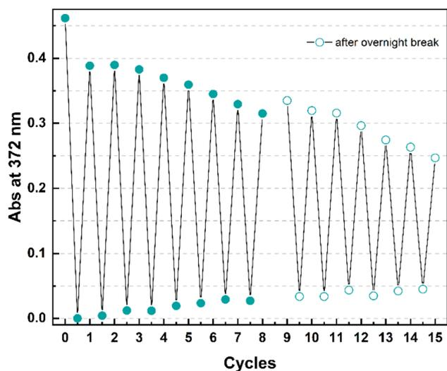
Fig. 8 Cyclability study for **4** in mesitylene showing the absorption change at 372 nm upon 15 irradiation (365 nm, 2 min) – heating (130 °C, 1 h) cycles. After the 8th cycle, the experiment was stopped. A gap is present between cycles 8 and 9 because the overnight break led to some evaporation which required the addition of fresh mesitylene to re-adjust the concentration before the restart of the experiment.
