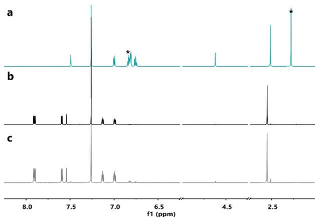
Fig. 5  $^1\text{H-NMRs}$  in  $\text{CDCl}_3$  of (a, blue-green solid line) **4c** after irradiation at 365 nm in non-degassed mesitylene; (b, black solid line) **4o** before irradiation at 365 nm in non-degassed mesitylene; and (c, grey solid line) recovered **4o** after the DSC measurement. \*: peaks of residual mesitylene.
