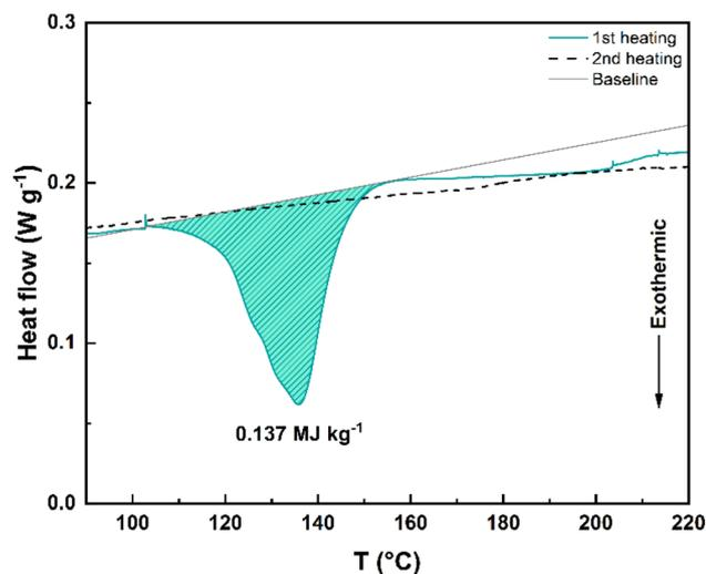
Fig. 4 DSC graph of **4c** showing the heat release during the first heating cycle (blue-green solid line). No heat release was observed during the second heating cycle (black dashed line). The baseline used for the integration to determine the energy release is provided with a solid grey line for clarity.
