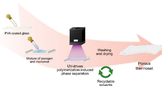
Fig. 2 Process schematic of thermoset membrane fabrication.
