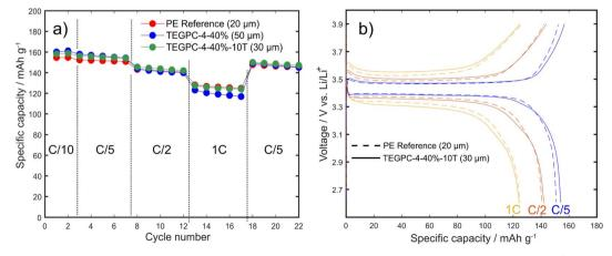
Fig. 10 Cycling performance of LFP/Li half cells cycled from 2.6 to 3.9 V at 22 °C (cathode mass loading = 13.3 mA h g<sup>-1</sup>). (a) Capacity retention test at different C-rates with 1C = 150 mA g<sup>-1</sup>. (b) Voltage vs. specific capacity at different C-rates, the final cycle of each step was taken (cycle 7, 12 and 17).
