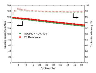
Fig. 11 Cycling performance of LFP/Li half cells using a TEGPC-4-40%-10T separator (green) or PE reference (red), cycled from 2.6 to 3.9 V at 22 °C. Two formation cycles at C/10 were followed by 50 cycles at C/5
