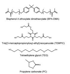
Fig. 1 Molecular structures of monomers and porogens used in the present study
