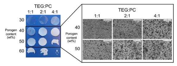
Fig. 4 (Left) Digital photographs of different porous membranes made using varying contents the porogens TEG and PC. (Right) Cross-sectional SEM micrographs of the freeze fractured films of selected formulations, showing a variation in pore size.
