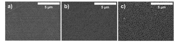
Top view SEM micrographs of the surface of (a) PE reference material (b) TEGPC-2-40% and (c) TEGPC-4-40% at 10 000× magnification.
