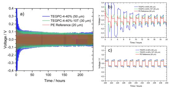
Fig. 9 Voltage profiles of Li/Li symmetrical cell cycling at 0.5 mA cm<sup>-1</sup> (0.5 mA h cm<sup>-1</sup>) with PE reference and two thermoset membrane formulations for (a) first 240 hours, (b) first 20 hours and (c) hours 220–240. The cells were stopped after 245 hours.
