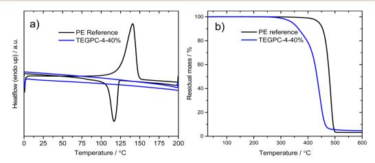
Fig. 6 (a) DSC thermograph with a heating rate of 10 °C min<sup>-1</sup> and cooling rate of 5 °C min<sup>-1</sup> and (b) TGA thermograph with a heating rate of 10 °C min<sup>-1</sup> C min<sup>-1</sup> of a representative thermoset membrane.
