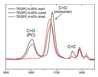
Fig. 3 FTIR spectra of TEGPC-4-40% before and after curing, and after washing and drying the membrane. The peak at 1637 cm<sup>-1</sup> represents the vinyl stretching mode. The peak at 1800 cm<sup>-1</sup> represents the carbonyl stretching on PC.
