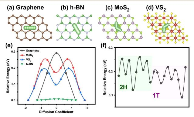
Fig. 5 Potential energy profile of Li atom diffusion on the surfaces. Top views of the optimized Li atom diffusion pathways on (a) graphene, (b) h-BN, (c) MoS<sub>2</sub> and (d) VS<sub>2</sub>. (e) Comparison of Li diffusion barrier of graphene, MoS<sub>2</sub>, VS<sub>2</sub> and h-BN and (f) between 2H and 1T transition metal sulfides and selenides.
