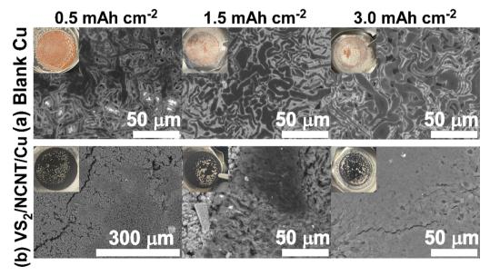
Fig. 7 Investigations of Li electrodeposition behaviors. The morphology of Li plating by SEM on (a) blank Cu and (b)  $VS_2/NCNT/Cu$  with the capacity of  $0.5 \text{ mA h cm}^{-2}$ ,  $1.5 \text{ mA h cm}^{-2}$  and  $3.0 \text{ mA h cm}^{-2}$  at  $10 \text{ mA cm}^{-2}$ . The insets are the optical images of the disassembled electrode after the Li plating process. Li deposition on VS<sub>2</sub>/NCNT/Cu is smooth and compact, without the dendrite formation.
