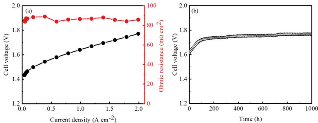
Fig. 11 Water electrolysis cell performance and ohmic resistance (a) and durability at a constant current density of  $1.0 \text{ A cm}^{-2}$  (b) for the AEMWE cell assembled with the  $\text{C}_{11}$ -QPip-1.86 membrane with 1 M KOH using  $\text{Ni}_{0.8}\text{Co}_{0.2}\text{O}$  (anode) and Pt/C (cathode) catalysts at  $80^\circ\text{C}$ .
