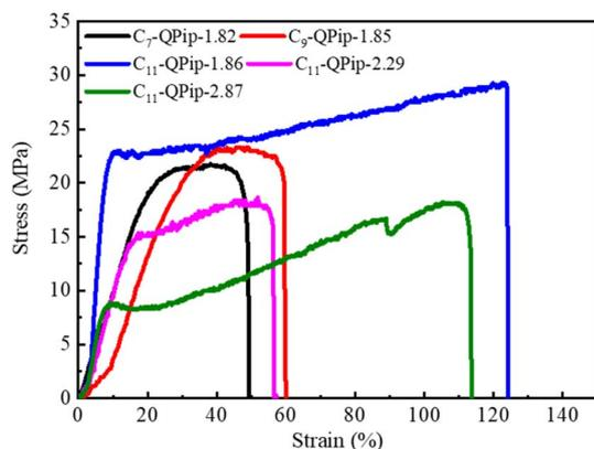
Fig. 8 Stress versus strain curves for  $C_7$ -QPip-1.82,  $C_9$ -QPip-1.85, and  $C_{11}$ -QPip- $n$  membranes in the chloride counter anion form at 60% RH and 80 °C.
