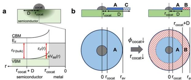
Fig. 4 A schematic illustration of the analytical model for prediction in the catalytic reactivity of CeO<sub>2</sub>: (a) a scheme of the calculation model of the cocatalyst-loaded CeO<sub>2</sub> to calculate the surface reaction rate; (b) two cases of depletion region formation on the CeO<sub>2</sub> surface. The blue color area is the depletion region (band bending area, A), and the red color area is the area where cocatalyst loading does not affect the Fermi level.
