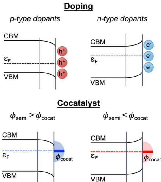
Fig. 1 Schematic illustration of surface Fermi level modification strategies: doping and cocatalyst.
