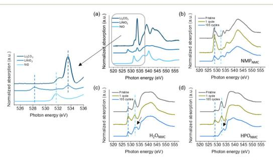
Fig. 8 O K-edge data in TEY mode for (a) reference materials including Li<sub>2</sub>O<sub>3</sub>, LiNiO<sub>2</sub>, and NiO. (b) NMP<sub>NMC</sub> electrodes, (c) H<sub>2</sub>O<sub>NMC</sub> electrodes, and (d) HPO<sub>NMC</sub> electrodes as pristine, after the 1 cycle, and after 105 cycles.
