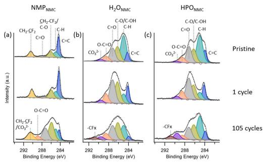
Fig. 2 C 1s spectra collected on NMP $_{NMC}$  (a),  $H_2O_{NMC}$  (b), and HPO $_{NMC}$  (c) electrodes as pristine (top) in the discharge state after the initial cycle (middle) and after 105 cycles (bottom) with photon energy 425 eV
