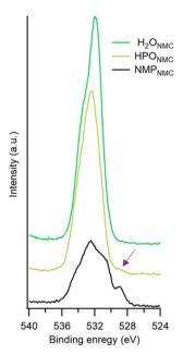
Fig. 4 O 1s spectra measured on  $NMC_{NMP}$ ,  $H_2O_{NMC}$  and  $HPO_{NMC}$  electrodes after 105 cycles with photon energy 1486.7 eV.
