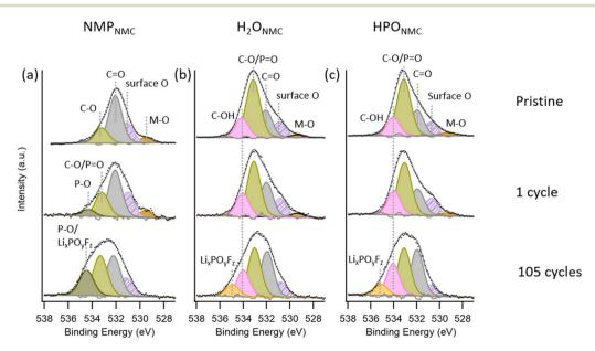
Fig. 3 O 1s spectra collected on NMP<sub>NMC</sub> (a), H<sub>2</sub>O<sub>NMC</sub> (b), and HPO<sub>NMC</sub> (c) electrodes as pristine (top), after 1 cycle (middle) and after 105 cycles (bottom) with photon energy 675 eV.
