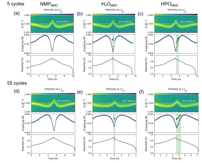
Operando synchrotron XRD characterization of 003 reflection of NMP<sub>NMC</sub> (a and d), NMC\_ H<sub>2</sub>O (b and e), and HPO<sub>NMC</sub> (c and f) electrodes after 5 formation cycles and 55 cycles along with the cycling profile at 0.5C.
