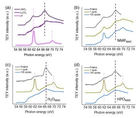
Fig. 7 Li K-edge data in TEY mode for (a) reference materials including LiNiO<sub>2</sub>, Li<sub>2</sub>O<sub>3</sub>, and LiF. (b) NMP<sub>NMC</sub> electrodes, (c)  $H_2O_{NMC}$  electrodes, and (d) HPO<sub>NMC</sub> electrodes as pristine, after the 1 cycle, and after 105 cycles.
