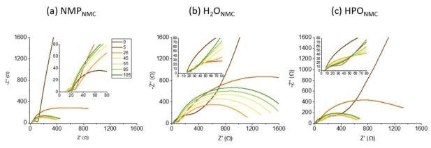
Fig. 11 EIS measurements of (a) NMP<sub>NMC</sub>, (b)  $H_2O_{NMC}$ , and (c) HPO<sub>NMC</sub> electrodes after various cycles.
