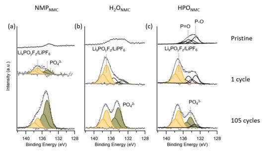
Fig. 5 P 2p spectra collected on NMP<sub>NMC</sub> (a),  $H_2O_{NMC}$  (b), and  $HPO_{NMC}$  (c) electrodes as pristine (top), after 1 cycle (middle), and after 105 cycles (bottom) with photon energy 275 eV.
