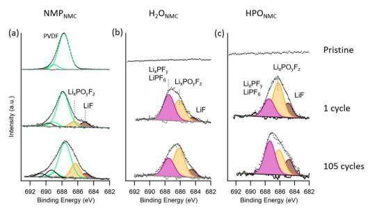
Fig. 6 F 1s spectra collected on NMP<sub>NMC</sub> (a),  $H_2O_{NMC}$  (b), and HPO<sub>NMC</sub> (c) electrodes as pristine (top), after 1 cycle (middle) and after 105 cycles (bottom) with photon energy 820 eV.
