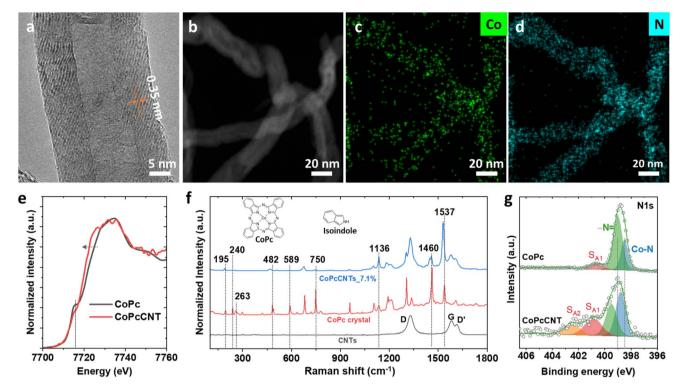
Fig. 1 (a) HRTEM image, (b) scanning transmission electron microscopy image and the (c and d) corresponding elemental maps of Co and N of as-synthesized CoPcCNT\_7.0%. (e) Co K-edge XANES spectra of CoPcCNT\_7.0% and bulk CoPc crystals. (f) Raman spectra of CoPcCNT\_7.0%, bulk CoPc crystals, and CNTs. (g) N 1s XPS spectra of bulk CoPc crystals and as-synthesized CoPcCNT\_7.0%.
