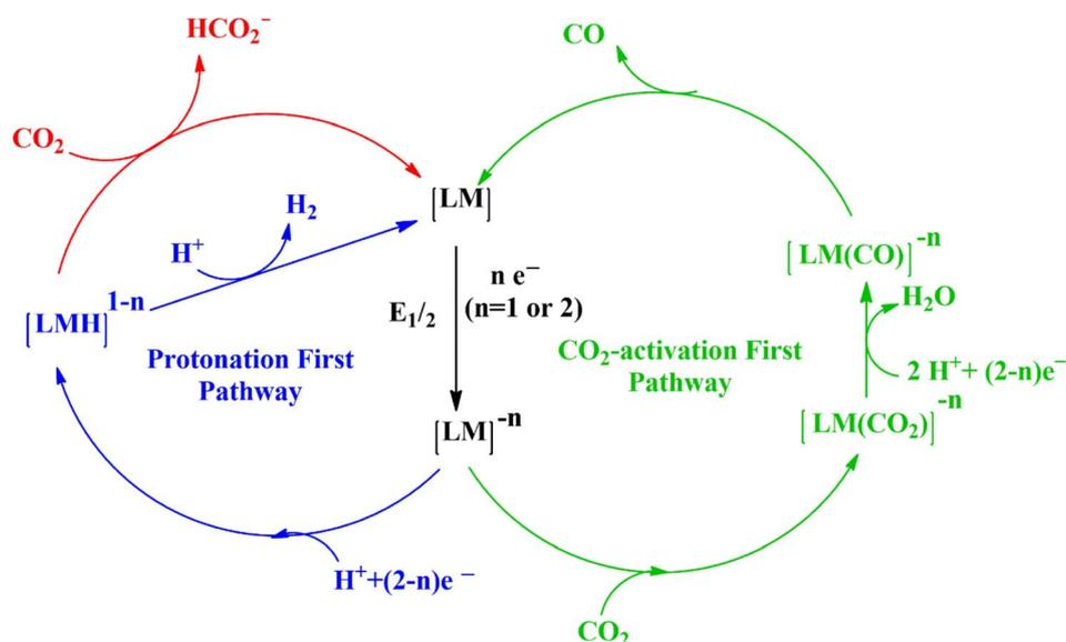
Scheme 1 Generalized scheme for CO<sub>2</sub> activation using molecular catalysts (M = metal, L = ligand, and n = charge).<sup>268</sup>
