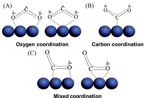
Fig. 2 Illustration of the possible orientation of  $\text{CO}_2$  on the surface of the electrocatalyst. (a) Oxygen coordination, (b) carbon coordination, (c) mixed coordination. Reproduced with permission.<sup>57</sup> Copyright 2016, the Royal Society of Chemistry.
