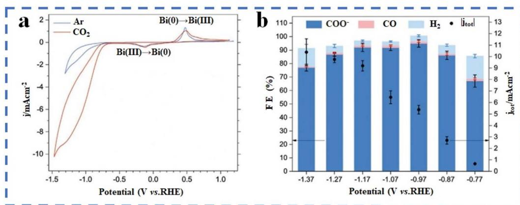
Fig. 11 (a) Multiple cycling of the  $\text{Bi}^{3+}/\text{Bi}^0$  redox couple under Ar and  $\text{CO}_2$ . (b) Faradaic efficiency of the electrocatalysis products at different potentials. Reproduced with permission.<sup>260</sup> Copyright 2020, Wiley-VCH.
