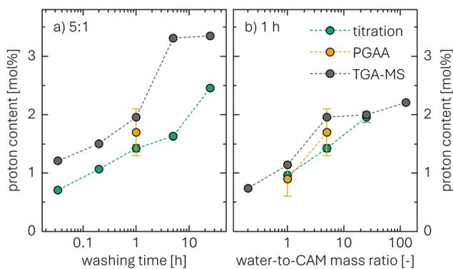
Fig. 8 Summary of the obtained proton content  $x_{\text{H}^+}$  for the two measurement series: (a) with a water-to-CAM mass ratio of 5:1 as a function of washing time, and (b) for a washing time of 1 h as a function of the water-to-CAM mass ratio. Note that the x-axes are plotted in a logarithmic representation. The data are extracted from Table 1 for the titration technique (green circles), from Table 2 for PGAA (yellow symbols), and from Table 3 for TGA-MS (gray symbols).
