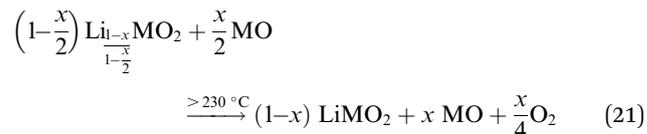
Note that despite the different intermediate phases, the sum of eqn (20) and (21) results in the same overall reaction as the sum of eqn (16) and (17), so that the above proposed TGA-MS analysis of the proton content is valid (see eqn (19)), irrespective of the intermediate phases.
