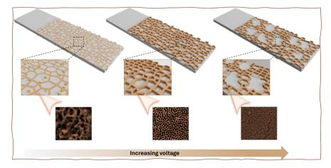
Scheme 1 Schematic illustrates an anodic oxidation process at different voltages, such as 65 V, 75 V, and 85 V, carried out on the cost-effective stainless steel (SS) 304, primarily containing iron (Fe), chromium (Cr), and nickel (Ni). Anodizing SS with ethylene glycol and ammonium fluoride electrolytes involves electrochemical reactions, complex formation processes, dissolution processes, and oxide growth mechanisms, forming a protective and functional nano-porous oxide layer.
