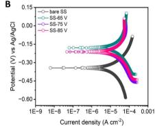
Fig. 5 Corrosion testing of anodized SS electrodes. (A and B) Potentiodynamic polarization curves for bare and anodized SS corrosion testing in (A) 3.5% NaCl and (B) 1 M KOH solution.
