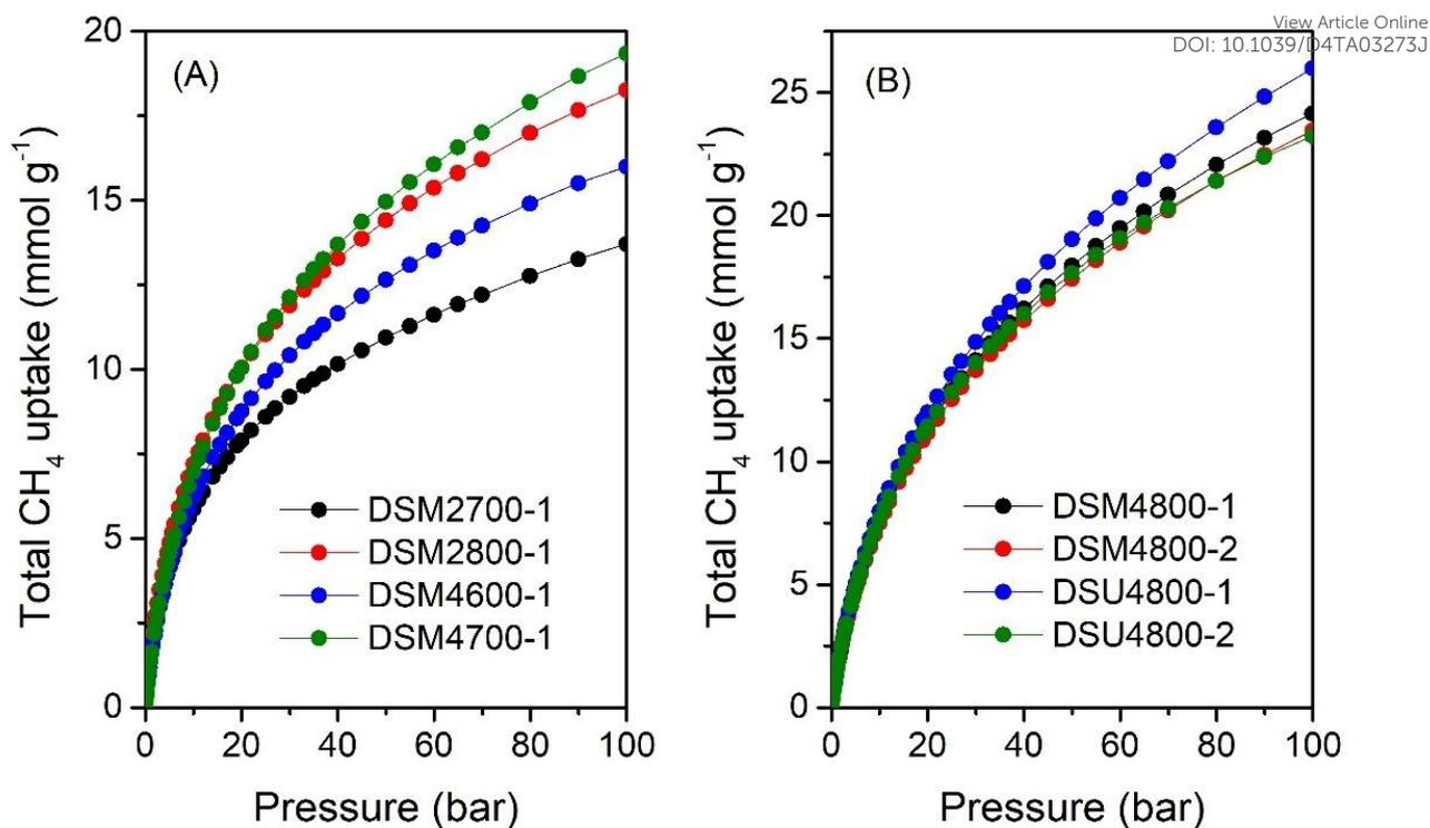
Figure 10. Total gravimetric methane uptake at 25 °C of N-doped activated carbons prepared at KOH/ACDS ratio of 2 or 4 and melamine or urea/ACDS ratio of 1 or 2.
