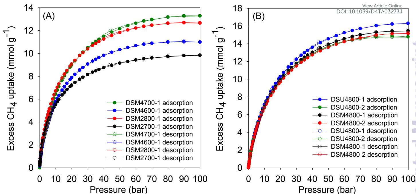
Figure 9. Excess gravimetric methane uptake at 25 °C of N-doped activated carbons prepared at KOH/ACDS ratio of 2 or 4 and melamine or urea/ACDS ratio of 1 or 2.
