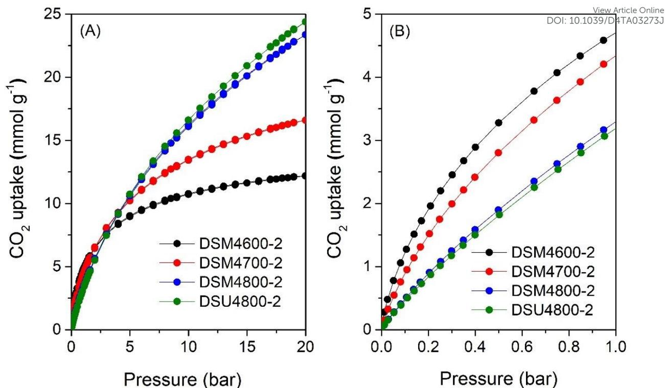
Figure 8. CO<sub>2</sub> uptake at 25 °C of N-doped activated carbons prepared at melamine or urea/ACDS ratio of 2 and KOH/ACDS ratio of 4.
