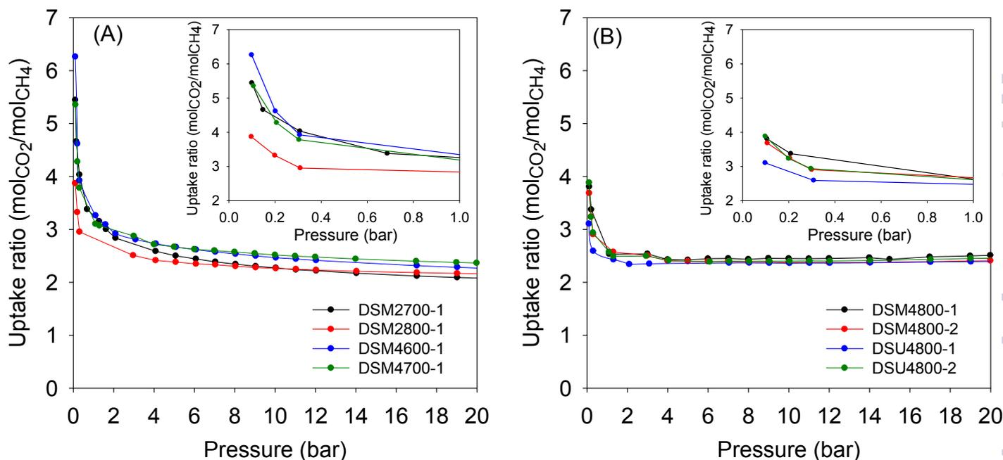
Figure 12. Uptake ratio of CO<sub>2</sub>/CH<sub>4</sub> as a function of pressure for a 50/50 mix of the gases.
