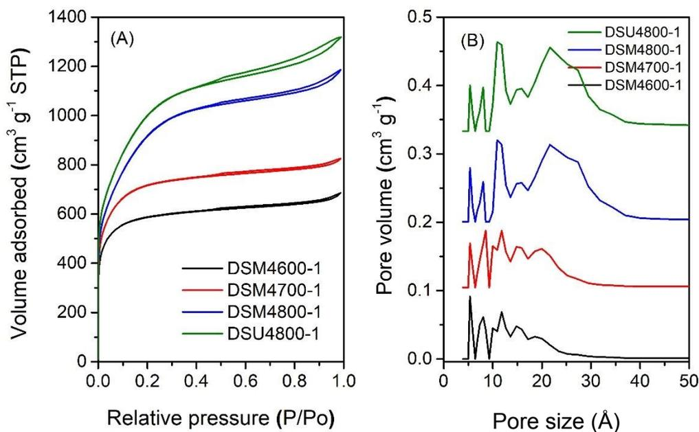
Figure 2. Nitrogen sorption isotherms (A) and pore size distribution curves (B) of activated carbons prepared at melamine or urea/ACDS ratio of 1 and KOH/ACDS ratio of 4.
