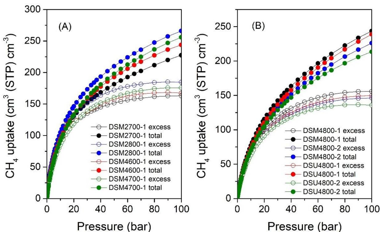
Figure 11. Excess and total volumetric methane uptake isotherms at 25 °C of N-doped activated carbons prepared at KOH/ACDS ratio of 2 or 4 and melamine or urea/ACDS ratio of 1 or 2.
