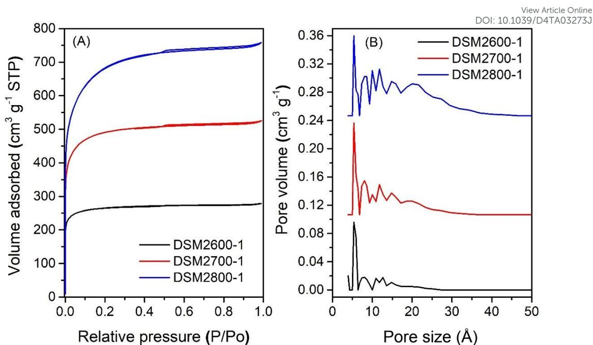
Figure 1. Nitrogen sorption isotherms (A) and pore size distribution curves (B) of activated carbons prepared at melamine/ACDS ratio of 1 and KOH/ACDS ratio of 2.
