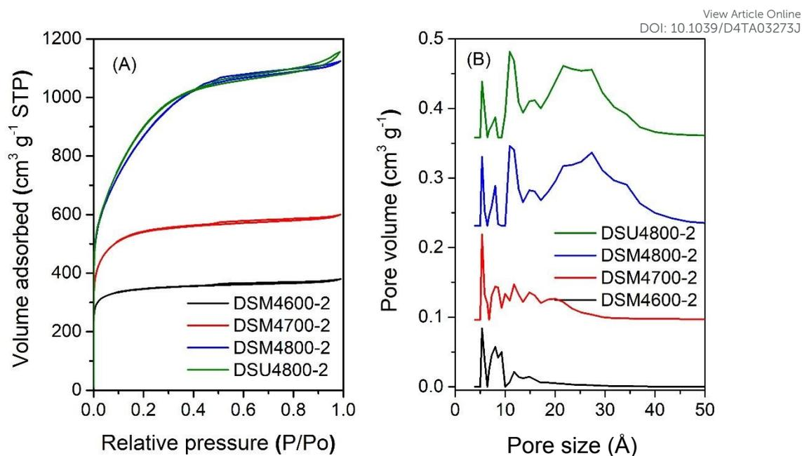
Figure 4 Nitrogen sorption isotherms (A) and pore size distribution curves (B) of activated carbons prepared at melamine or urea/ACDS ratio of 2 and KOH/ACDS ratio of 4.
