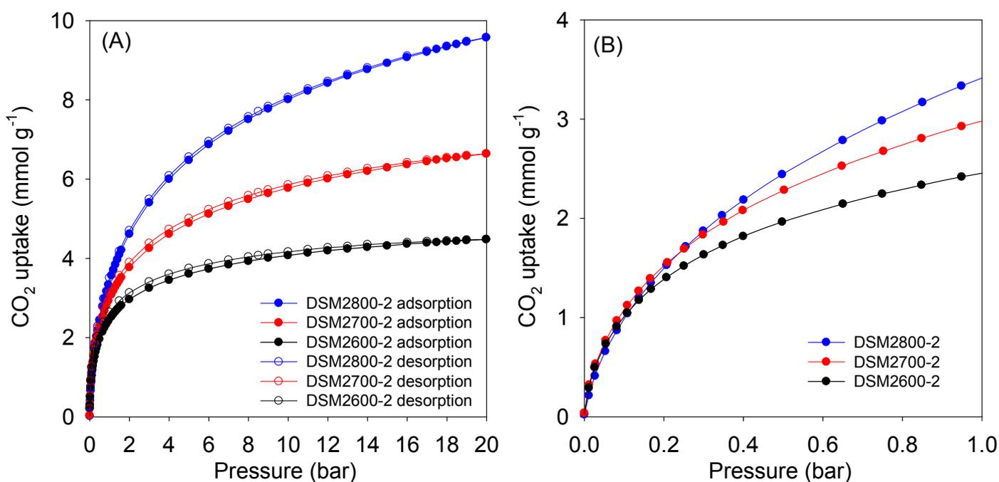
Figure 7. CO<sub>2</sub> uptake at 25 °C of N-doped activated carbons prepared at melamine/ACDS ratio of 2 and KOH/ACDS ratio of 2.
