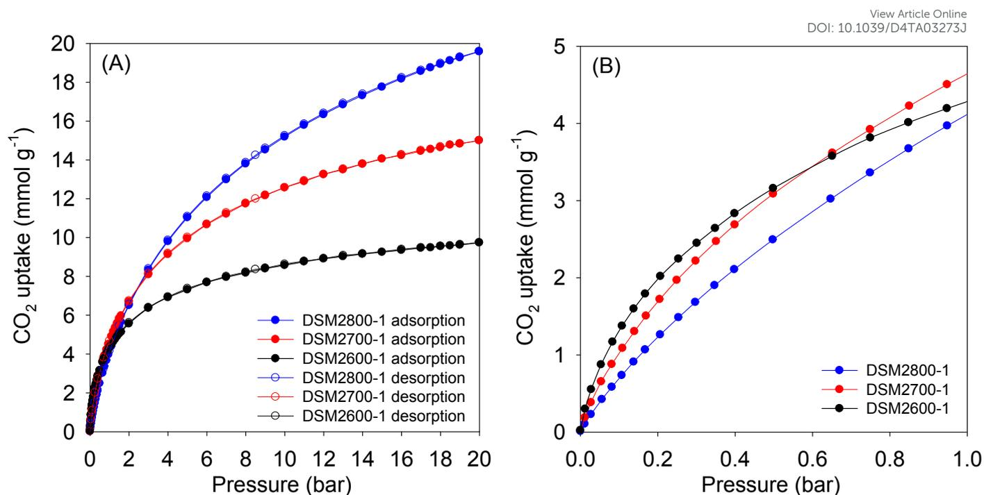
Figure 5. CO<sub>2</sub> uptake at 25 °C of N-doped activated carbons prepared at melamine/ACDS ratio of 1 and KOH/ACDS ratio of 2.
