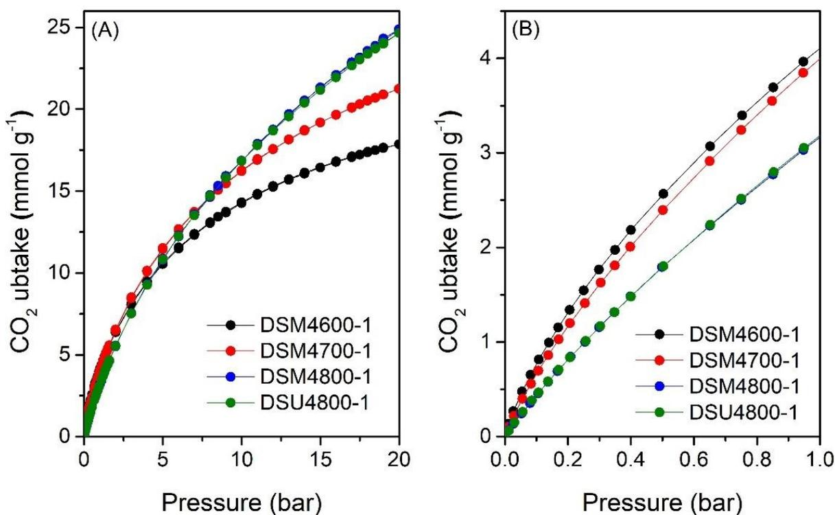
Figure 6. CO<sub>2</sub> uptake at 25 °C of N-doped activated carbons prepared at melamine or urea/ACDS ratio of 1 and KOH/ACDS ratio of 4.
