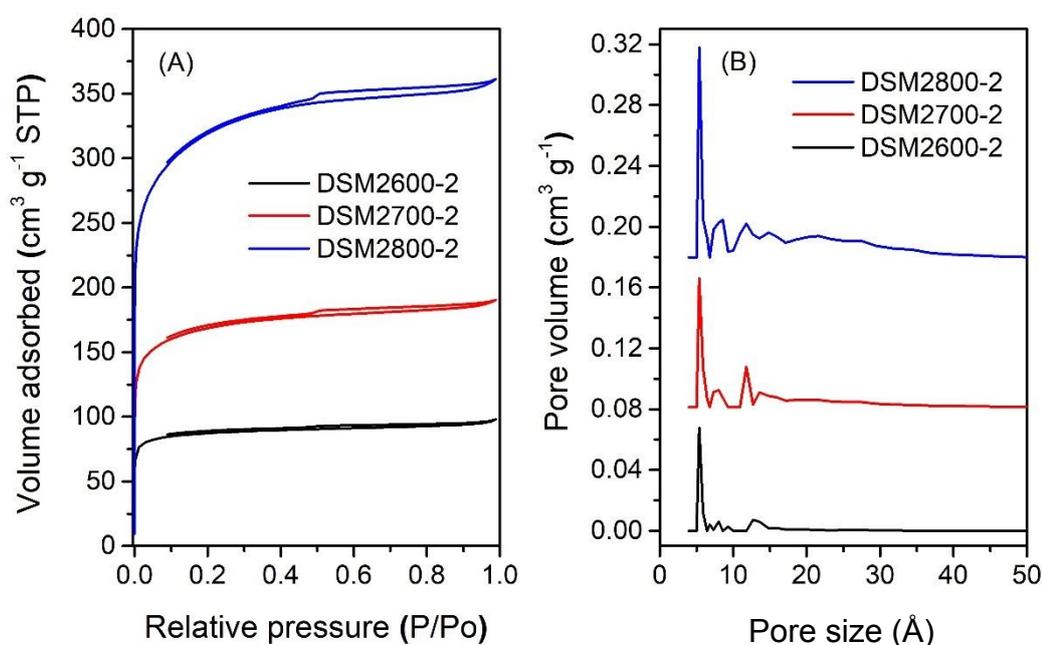
Figure 3. Nitrogen sorption isotherms (A) and pore size distribution curves (B) of activated carbons prepared at melamine/ACDS ratio of 2 and KOH/ACDS ratio of 2.
