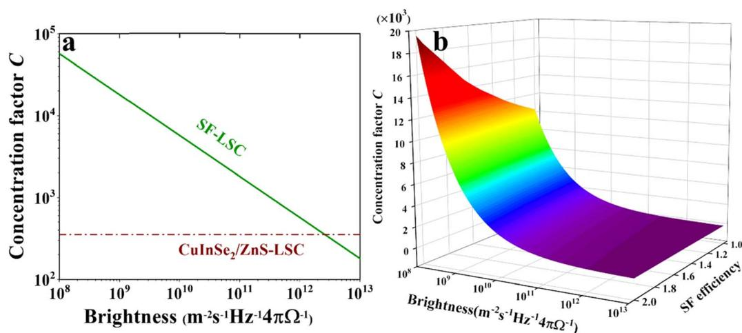
Fig. 5 (a) Thermodynamic limits of concentration factor  $C$  for NaGdF<sub>4</sub>:Yb-tetracene NC-based LSCs (green line) and CuInSe<sub>2</sub>/ZnS QD-based LSCs (red dash line) at room temperature. (b) Thermodynamic limits of concentration factor  $C$  as a function of SF efficiency and input brightness for NaGdF<sub>4</sub>:Yb-tetracene NC-based LSCs.
