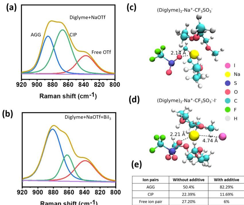
Fig. 1 Raman spectra of solvation shell (a) reference electrolyte and (b) with additive ions, (c and d) model structure of the population of different ion pairs in the solvation shell of the electrolyte without an additive and with an additive, and (e) calculated relative distribution of different ion pairs in the electrolyte with and without an additive. The model structure of the solvation shell consists of one diglyme molecule and  $\text{Na}^+$  ion.
