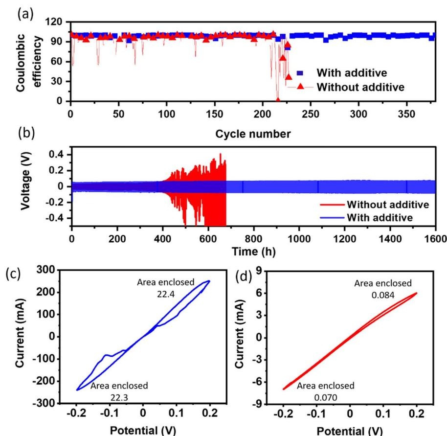
Fig. 4 (a) Coulombic efficiency of Na//Cu half cells with and without an additive at  $1 \text{ mA cm}^{-2}$  current density and  $1 \text{ mA h cm}^{-2}$  capacity. (b) Stripping plating cycling performance of a Na//Na symmetric cell at  $1 \text{ mA cm}^{-2}$  current density and  $1 \text{ mA h cm}^{-2}$  capacity, and the cyclic voltammogram of a Na//Na symmetric cell (c) with and (d) without an additive. The CV scans were conducted at a sweep rate of  $5 \text{ mV s}^{-1}$ .
