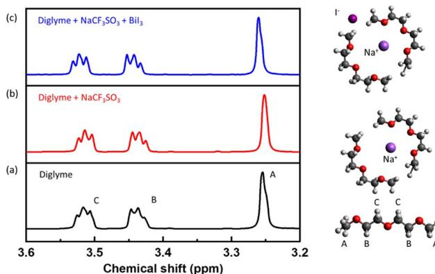
Fig. 2  $^1\text{H}$  NMR spectra of (a) pure diglyme solvent, (b) diglyme with sodium salt ( $\text{NaCF}_3\text{SO}_3$ ), and (c) diglyme with sodium salt ( $\text{NaCF}_3\text{SO}_3$ ) and additives ( $\text{BiI}_3$ ). Deuterated DMSO is used as the reference solvent for all three testing studies.
