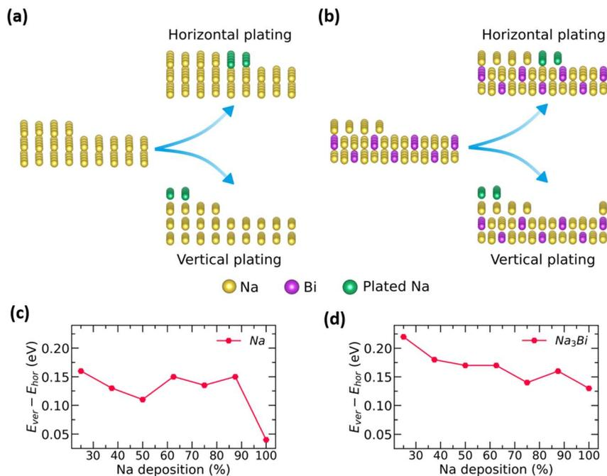
Fig. 5 Schematic representation illustrating the horizontal and vertical plating mechanisms of Na on (a) bulk Na-metal and (b)  $\text{Na}_3\text{Bi}$  surfaces. The graphs below show the variation in the energy difference between vertical and horizontal plating in response to varying Na deposition concentrations for (c) bulk Na-metal and (d)  $\text{Na}_3\text{Bi}$  surfaces.
