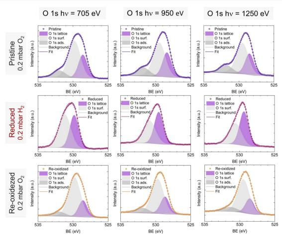
Fig. 5 NAP-XPS spectra of O 1s in the pristine (0.2 mbar  $O_2$ ), reduced (0.2 mbar  $H_2$ ), and re-oxidized (0.2 mbar  $O_2$ ) sample states recorded using three photon energies: 705, 950 and 1250 eV.
