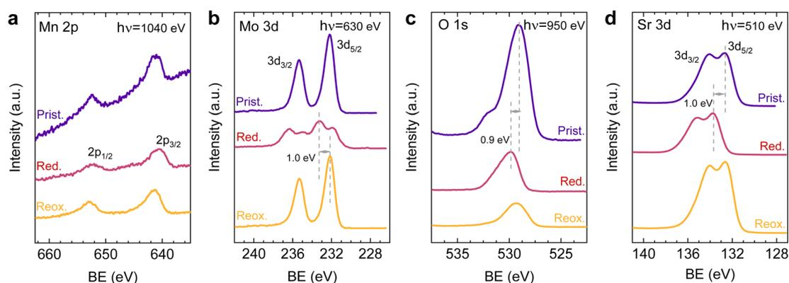
Fig. 4 NAP-XPS spectra of (a) Mn 2p, (b) Mo 3d, (c) O 1s, and (d) Sr 3d acquired *in situ* at 600 °C in pristine ("Prist.", 0.2 mbar  $\text{O}_2$ ), reduced ("Red.", 0.2 mbar  $\text{H}_2$ ) and re-oxidized ("Reox.", 0.2 mbar  $\text{O}_2$ ) conditions. The used photon energies (to result in a similar electron kinetic energy of ~400 eV) are indicated in the panels. A constant offset for better clarity is added to the spectra.
