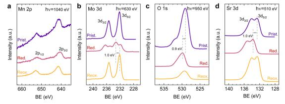
Fig. 4 NAP-XPS spectra of (a) Mn 2p, (b) Mo 3d, (c) O 1s, and (d) Sr 3d acquired *in situ* at 600 °C in pristine ("Prist.", 0.2 mbar  $O_2$ ), reduced ("Red.", 0.2 mbar  $H_2$ ) and re-oxidized ("Reox.", 0.2 mbar  $O_2$ ) conditions. The used photon energies (to result in a similar electron kinetic energy of  $\sim$ 400 eV) are indicated in the panels. A constant offset for better clarity is added to the spectra.
