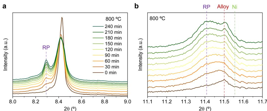
Fig. 9 Time-resolved *in situ* XRD at 800 °C, during the first reduction step in 5% H<sub>2</sub>/Ar for (a) the 8–9° region and (b) the 11.1–11.7° region, exhibiting the formation of the Ruddlesden–Popper phase (RP), the exsolution of ternary alloyed NPs and the emergence of Ni caused by the reduction of minor NiO impurities.
