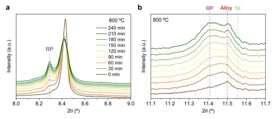
Fig. 9 Time-resolved in situ XRD at 800 °C, during the first reduction step in  $5\% H_2/Ar$  for (a) the 8-9° region and (b) the 11.1-11.7° region, exhibiting the formation of the Ruddlesden-Popper phase (RP), the exsolution of ternary alloyed NPs and the emergence of Ni caused by the reduction of minor NiO impurities.
