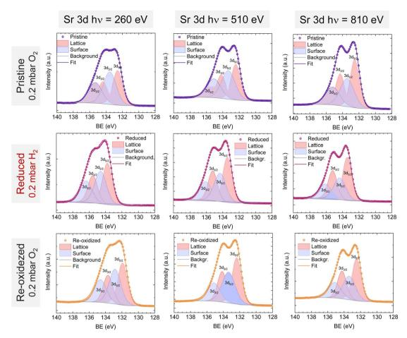
Fig. 6 NAP-XPS spectra of Sr 3d at the pristine  $(0.2 \text{ mbar } O_2)$ , reduced  $(0.2 \text{ mbar } H_2)$ , and re-oxidized  $(0.2 \text{ mbar } O_2)$  sample states recorded using three photon energies: 260, 510, and 810 eV.
