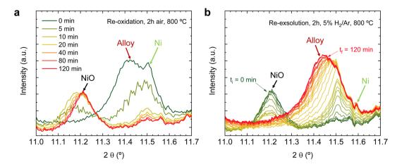
Fig. 10 Time-resolved in situ XRD at 800 °C, during (a) the re-oxidation step of 2 h under air atmosphere followed by (b) the second reduction step in 5% H<sub>2</sub>/Ar for the region between 11.1 and 11.7°.
