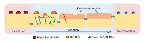
Fig. 12 Schematic representation of the ex situ redox processes affecting the exsolved NPs in  $Sr_2FeCo_{0.2}Ni_{0.2}Mn_{0.1}Mo_{0.5}O_{6-\delta}$ , and their latter redissolution and re-exsolution.
