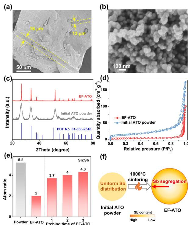
Fig. 1 The structural properties of EF-ATO. (a and b) SEM images. (c) XRD patterns. (d) N<sub>2</sub> adsorption–desorption isotherms. The initial ATO powder is shown for comparison. (e) Surface Sn : Sb atomic ratio and in-depth Sn : Sb from XPS. (f) Illustration of heat-driven Sb segregation in EF-ATO.
