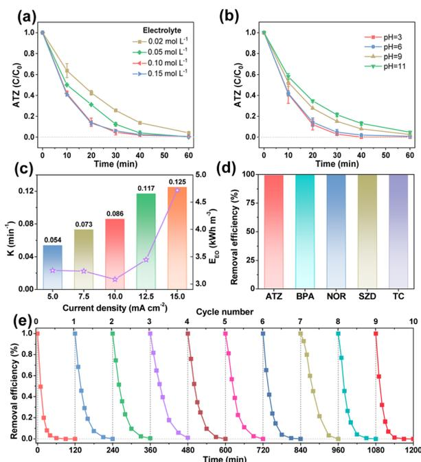
Fig. 3 Influence factors of ATZ removal on EF-ATO anode. Removal efficiency under a series of electrolyte (a) concentration and (b) pH. (c) Removal rate constant and  $E_{EO}$  at a series of current densities. (d) Removal efficiency of different pollutants. (e) Recyclability of EF-ATO anode for ATZ removal. If not specified, experimental conditions:  $C_0 = 20 \text{ mg L}^{-1}$ ,  $j = 10 \text{ mA cm}^{-2}$ ,  $\text{pH} = 6$ , and  $\text{Na}_2\text{SO}_4$  concentration =  $0.1 \text{ M}$ .
