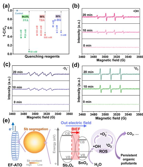
Fig. 4 ROS determination. (a) Quenching tests with TBA, FFA, and *p*-BQ, respectively. *In situ* EPR spectra of (b)  $\cdot\text{OH}$ , (c)  $\cdot\text{O}_2^-$ , and (d)  $^1\text{O}_2$ . (e) Illustration of EF-ATO with Sb segregation enhanced EO process for persistent organic pollutants removal.
