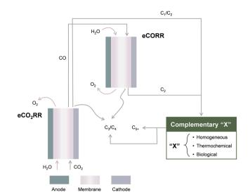
Fig. 1 Schematic illustration of direct electrochemical approaches (eCO<sub>2</sub>RR and eCORR) and "electrochemical + X" approaches for upgrading CO<sub>2</sub> to C<sub>3+</sub> products.
