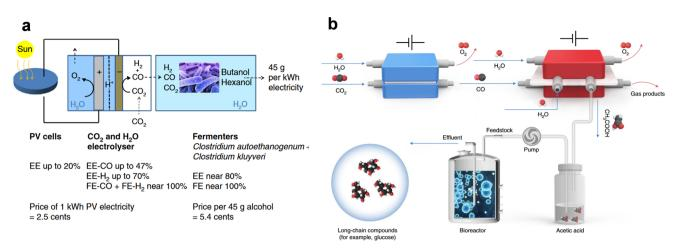
Fig. 9 "Electrochemical + biological" approaches. (a) Schematic illustration of the  $CO_2$  electrolyzer coupled to a fermentation module for the synthesis of 1-butanol and 1-hexanol. Adapted from ref. 139 with permission from Springer Nature. (b) Schematic illustration of the *in vitro* artificial sugar synthesis system based on the two-step  $eCO_2RR-eCORR$  and yeast fermentation. Adapted from ref. 33 with permission from Springer Nature.
