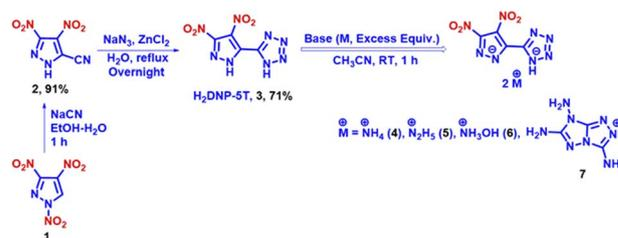
Scheme 3 Synthesis of **H<sub>2</sub>DNP-5T** (**3**) and its ionic derivatives, **4**, **5**, **6**, and **7**.
