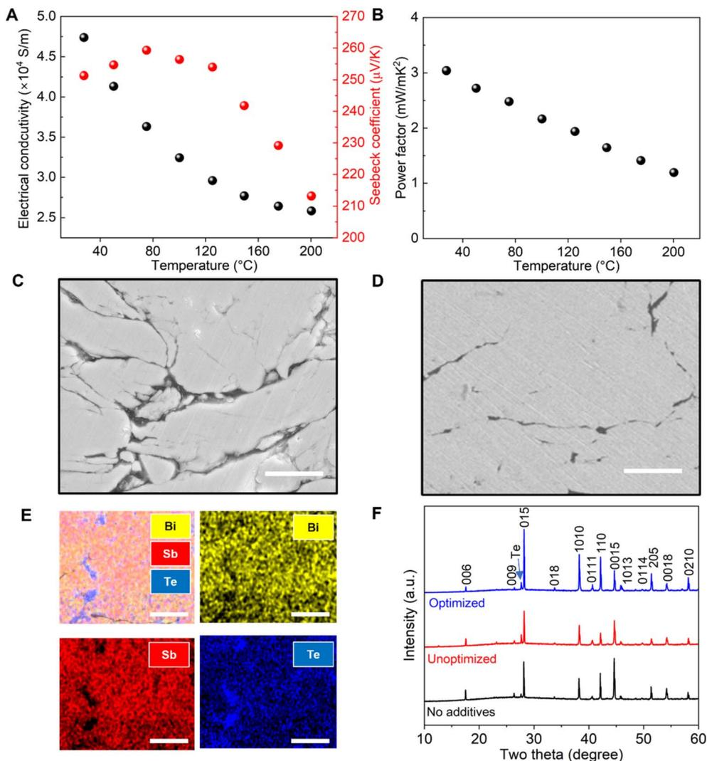
Fig. 3 (A and B) Temperature-dependent electrical conductivity, Seebeck coefficient, and power factor. (C and D) Scanning electron microscope (SEM) images of the cross-section of samples printed using unoptimized and optimized inks (scale bar 10  $\mu\text{m}$ ). (E) Elemental analysis of the sample printed using the optimized ink (scale bar 10  $\mu\text{m}$ ). (F) XRD of printed samples with and without X-gum rheological modifier.
