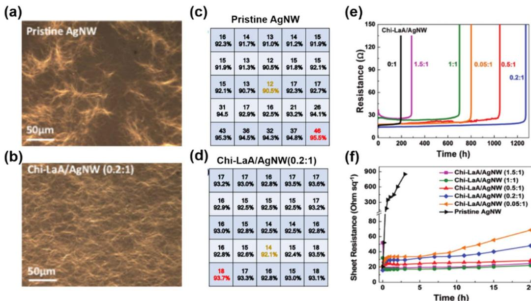
Fig. 3 The stability of the pristine Ag NW and uniform Chi-LaA/Ag NW FTEs. (a and b) Optical images. (c and d) Sheet resistance and transmittance of FTEs with a size of  $6 \times 6 \text{ cm}^2$ . (e) Resistance as a function of time under a current of  $250 \text{ mA cm}^{-2}$ . (f) Sheet resistance as a function of time at high temperature of  $180 \text{ }^\circ\text{C}$ . Reproduced with permission.<sup>71</sup> Copyright 2020, the Royal Society of Chemistry.
