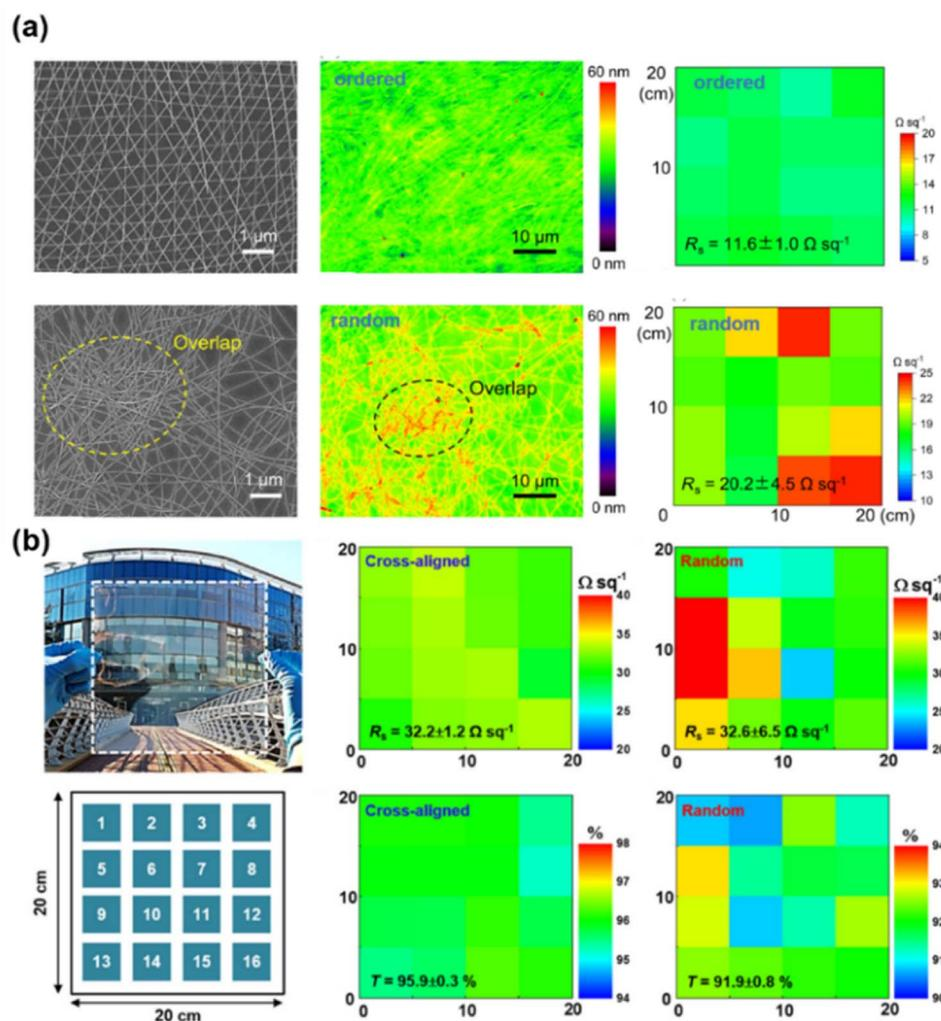
Fig. 5 Comparison of ordered and random Ag NW FTEs. (a) SEM images, AFM height profile, sheet resistance distribution. Reproduced with permission.<sup>101</sup> Copyright 2024, Wiley-VCH. (b) Photograph of large scale ( $20 \times 20 \text{ cm}^2$ ) FTE and the mapping showing the distribution of sheet resistance and transmittance for the cross-aligned and random Ag NW FTEs. Reproduced with permission.<sup>102</sup> Copyright 2017, American Chemical Society.
