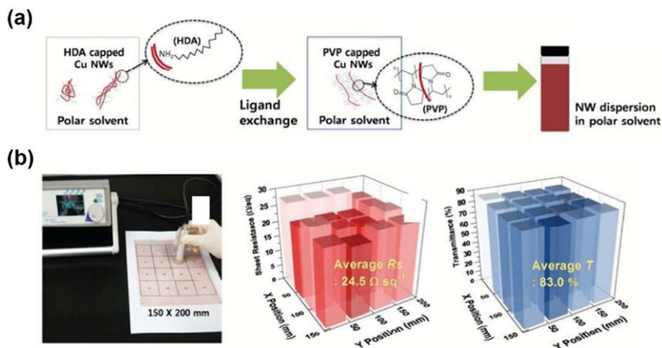
Fig. 6 Surface modification of Cu NWs for uniform FTEs. (a) Schematic illustration of the ligand exchange process for highly dispersed Cu NW ink. (b) Photograph of large-scale (150 × 200 mm<sup>2</sup>) Cu NW FTE divided into 16 zones to characterize its sheet resistance (center) and transmittance (right) uniformity. Reproduced with permission.<sup>109</sup> Copyright 2016, the Royal Society of Chemistry.
