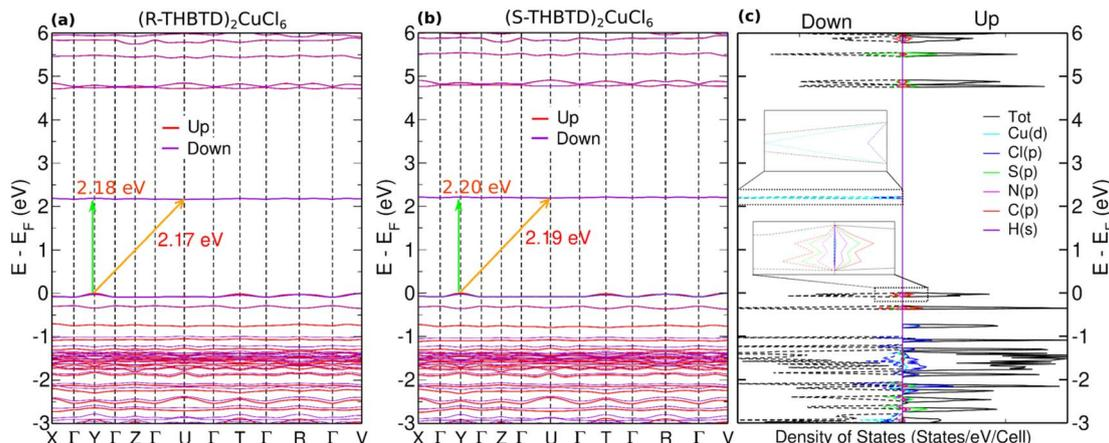
Fig. 3 Calculated band structures of the ferromagnetic phases of (a)  $(R\text{-THBTD})_2\text{CuCl}_6$  (b) and  $(S\text{-THBTD})_2\text{CuCl}_6$  materials, respectively. (c) Density of states of the  $(S\text{-THBTD})_2\text{CuCl}_6$  material, where the insets highlight an enlarged view of the PDOS that contributes to the VBM and CBM states. The spin-down and spin-up states are represented by a dashed line and a solid line, respectively.
