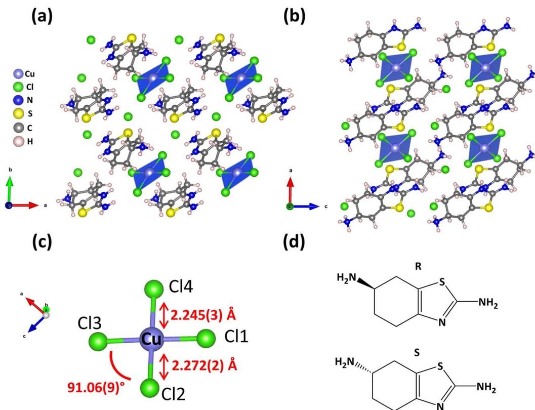
Fig. 1 Part of the crystal structure of (*R*-THBTD)<sub>2</sub>CuCl<sub>6</sub> viewed along the (a) *c*-axis and (b) *b*-axis, respectively. (c) Representation of the square planar geometry of the [CuCl<sub>4</sub>]<sup>2-</sup> moieties along with two representative Cu–Cl bond lengths and one Cl–Cu–Cl angle. (d) The molecular structures of the chiral ligands *S*-THBTD and *R*-THBTD.
