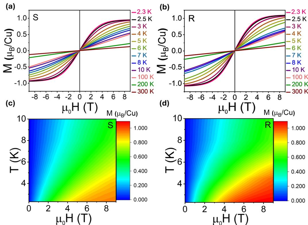
Fig. 7 Magnetic-field dependent magnetization ( $M$ – $H$ ) curves of (a)  $(S\text{-THBTD})_2\text{CuCl}_6$  and (b)  $(R\text{-THBTD})_2\text{CuCl}_6$  in a temperature range from 2.3 to 300 K; the 2D surface plots of change in magnetic moment with field and temperature for (c)  $(S\text{-THBTD})_2\text{CuCl}_6$  and (d)  $(R\text{-THBTD})_2\text{CuCl}_6$  for field changes up to 9 T and temperatures below 10 K.
