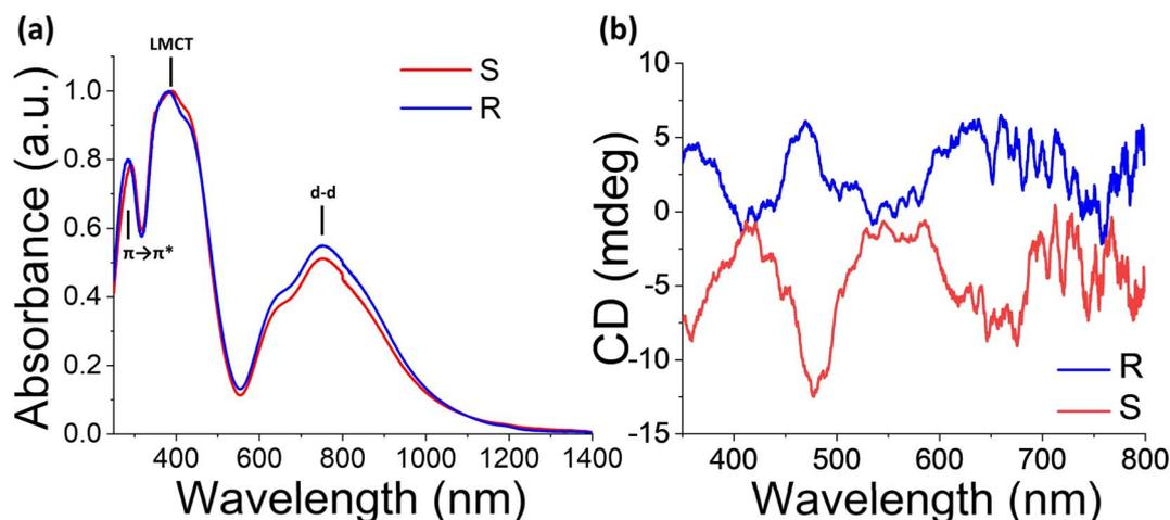
Fig. 4 (a) Comparison of normalized absorbance spectra for  $(R\text{-THBTD})_2\text{CuCl}_6$  and  $(S\text{-THBTD})_2\text{CuCl}_6$  along with the corresponding assigned transitions. (b) DRCD spectra for the  $(R\text{-THBTD})_2\text{CuCl}_6$  and  $(S\text{-THBTD})_2\text{CuCl}_6$  materials verifying their chiral nature.
