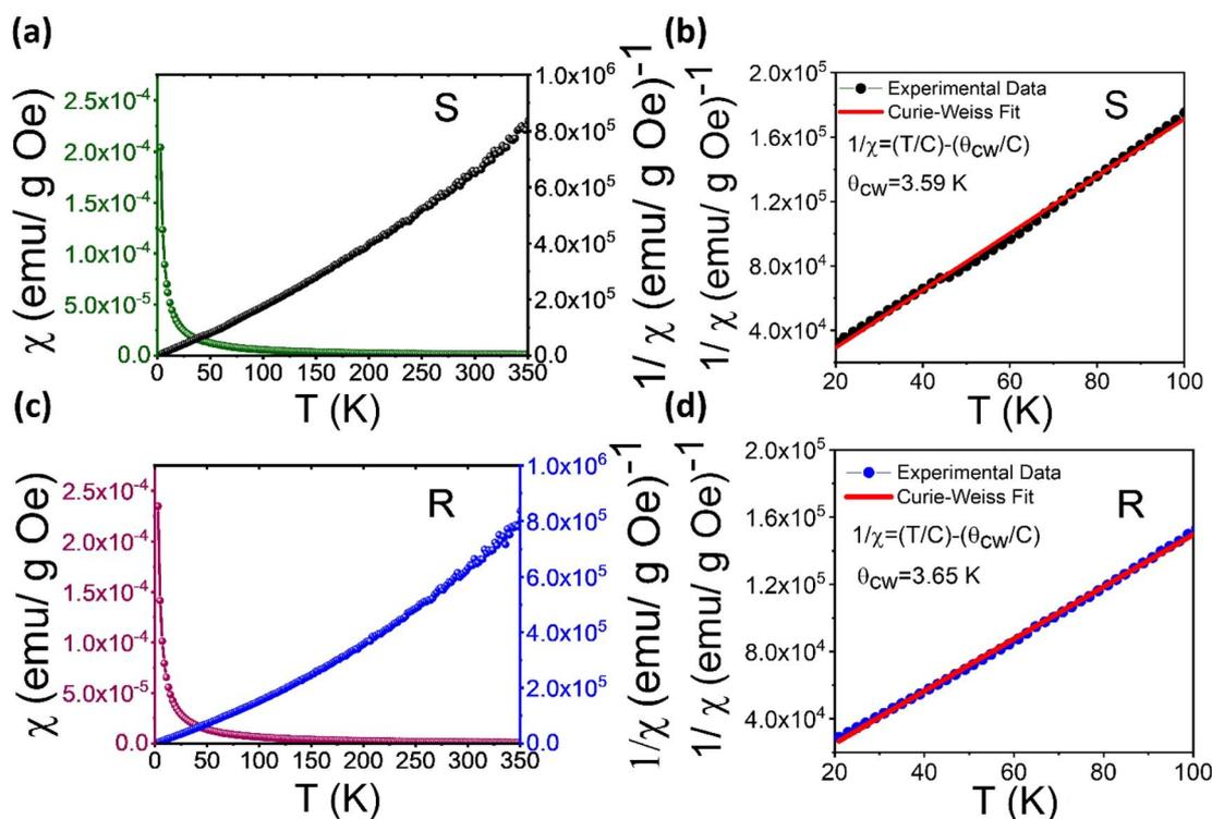
Fig. 5 Temperature-dependent magnetic susceptibility ( $\chi$ ) and inverse  $1/\chi$  under a 0.1 T static magnetic field of (a) (*S*-THBTD)<sub>2</sub>CuCl<sub>6</sub> and (c) (*R*-THBTD)<sub>2</sub>CuCl<sub>6</sub>; Curie-Weiss fit (red line) within the range of 20–100 K for (b) (*S*-THBTD)<sub>2</sub>CuCl<sub>6</sub> and (d) (*R*-THBTD)<sub>2</sub>CuCl<sub>6</sub>, respectively.
