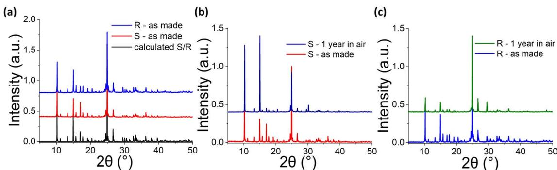
Fig. 2 (a) Comparison of the PXRD patterns for the as-made (*R/S*-THBTD)<sub>2</sub>CuCl<sub>6</sub> compounds to the calculated patterns derived from the solved single-crystal structure. (b) Comparison of the PXRD patterns for the *S* and (c) *R* enantiomers after 1 year of air exposure (RH = 35–55% ± 5%) to the calculated pattern derived from the solved single-crystal structure.
