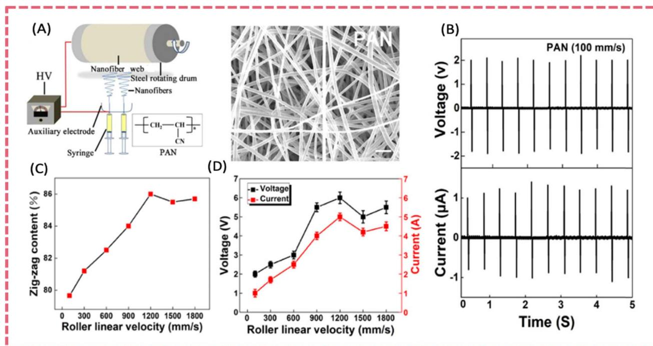
Fig. 7 (A) Electrospinning apparatus for producing PAN nanofiber membranes and SEM image of the as-spun PAN nanofibers. (B) Piezoelectric outputs of the nanofiber device under repeated compression impact (line speed 100 mm s<sup>-1</sup>, frequency 2 Hz). The effect of collector drum rotation speed on (C) planar zigzag conformation contents ( $\psi$ ) and (D) electric outputs of the energy devices. Reproduced from ref. 113 with permission from Elsevier, copyright 2019.
