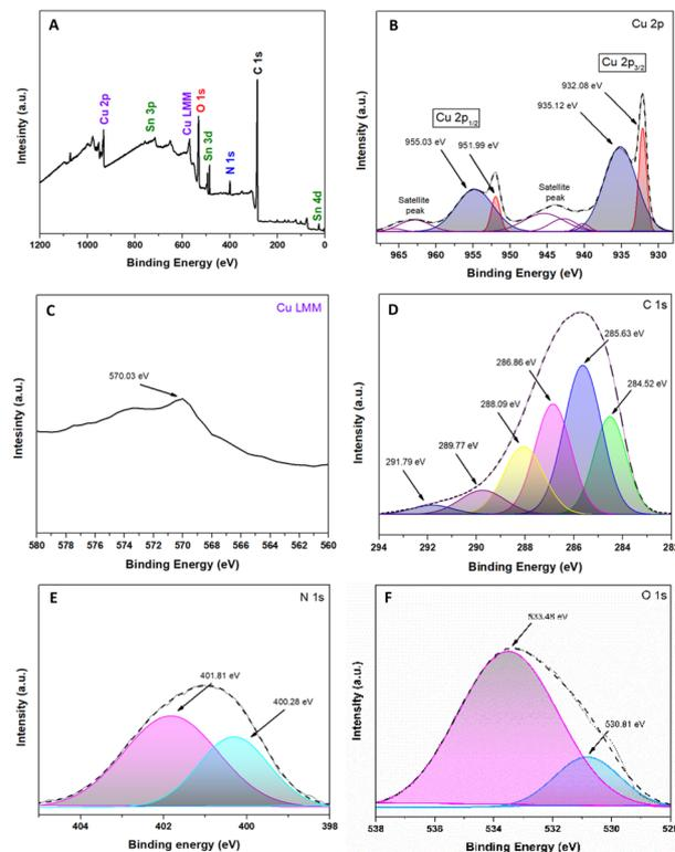
Fig. 4 Spectroscopic analysis XPS of the Cu<sub>2</sub>O@PCz electrode. (A) Survey spectra; (B) Cu 2p; (C) Cu 2p AES (Auger electron spectroscopy); (D) C 1s; (E) N 1s; and (F) O 1s.
