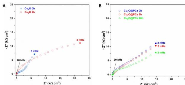
Fig. 11 Nyquist diagram of (A)  $\text{Cu}_2\text{O}$  and (B)  $\text{Cu}_2\text{O}@PCz$ , at different NRR times, using  $-0.6$  V (vs. Ag/AgCl).
