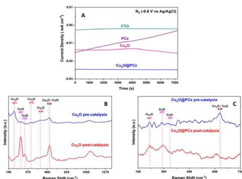
Fig. 9 Stability tests for the  $\text{Cu}_2\text{O}@PCz$  electrode and its components on applying a potential of  $-0.6$  V vs. Ag/AgCl in the presence of  $\text{N}_2$ : (A) galvanostatic curves for: FTO (green), PCz (purple),  $\text{Cu}_2\text{O}$  (pink), and  $\text{Cu}_2\text{O}@PCz$  (blue). (B) Raman spectra of the  $\text{Cu}_2\text{O}$  electrode before and after electrocatalysis. (C) Raman spectra of the  $\text{Cu}_2\text{O}@PCz$  electrode before and after electrocatalysis.
