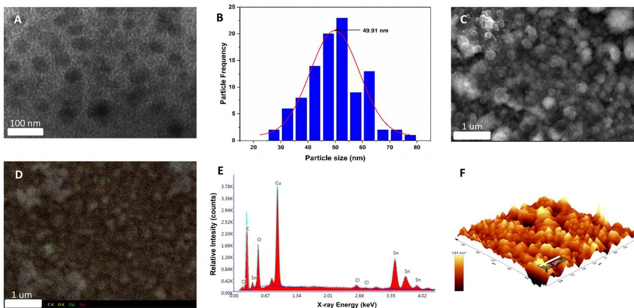
Fig. 1 Morphological and topographical characterization studies of the Cu<sub>2</sub>O@PCz electrode surface. (A) TEM image and (B) histogram of the size distribution of Cu<sub>2</sub>O nanoparticles on the Cu<sub>2</sub>O@PCz electrode surface. (C) FE-SEM image of the Cu<sub>2</sub>O@PCz electrode surface. (D) FE-SEM mapping of C, O, Cu and Sn. (E) EDX analysis and (F) AFM image of the Cu<sub>2</sub>O@PCz electrode surface.
