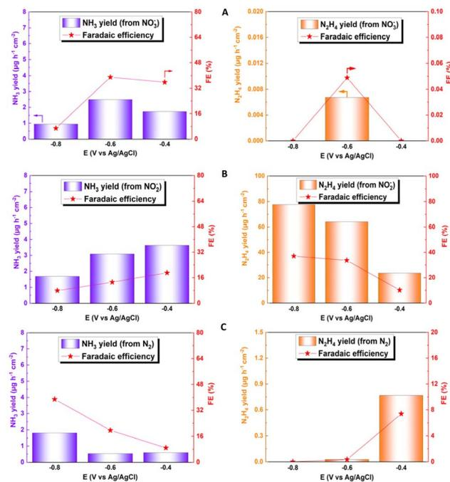
Fig. 6 Faradaic efficiency and generation rate at different potentials for ammonia (blue) and hydrazine (orange) for electroreduction of (A)  $\text{NO}_3^-$ , (B)  $\text{NO}_2^-$  and (C)  $\text{N}_2$ .
