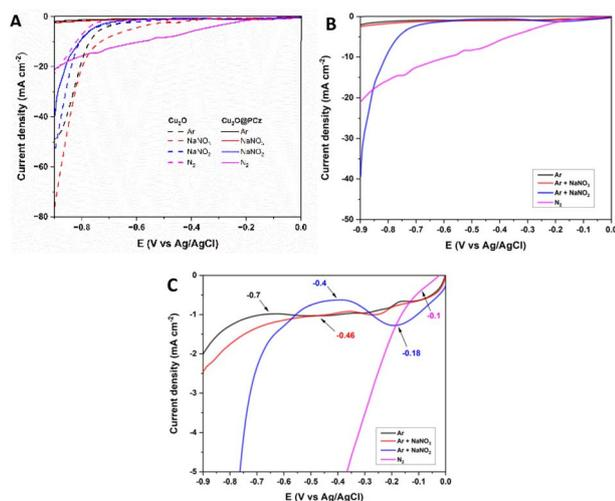
Fig. 5 (A) Polarization curve of  $\text{Cu}_2\text{O}$  and  $\text{Cu}_2\text{O}@PCz$  electrodes in the presence of different nitrogen species at  $1 \text{ mV s}^{-1}$ . (B) Separate  $\text{Cu}_2\text{O}@PCz$  polarization curves. (C) Magnification of the onset potential of  $\text{Cu}_2\text{O}@PCz$  curves.
