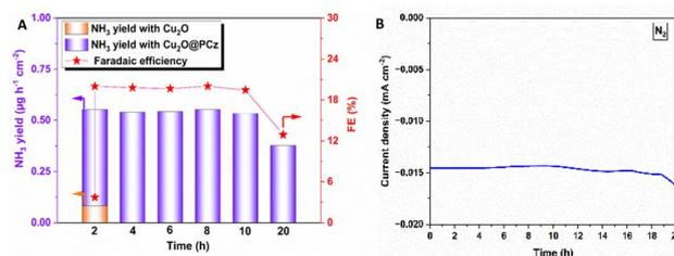
Fig. 8 (A) Faradaic efficiency and generation rate at different potentials for ammonia in the NRR process for 20 hours at  $-0.6 \text{ V}$  vs.  $\text{Ag}/\text{AgCl}$ . The two-hour bar shows a comparison between  $\text{Cu}_2\text{O}$  PCz-stabilized and  $\text{Cu}_2\text{O}$  non-stabilized electrodes. (B) Stability of the NRR process during 20 hours of electrolysis.
