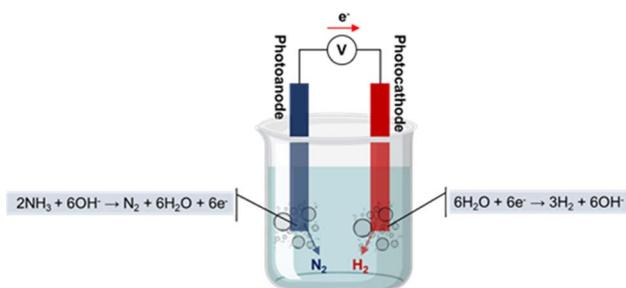
Fig. 3 Principle of electrolysis  $NH_3$  in aqueous solution for  $H_2$  production.
