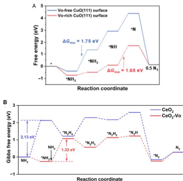
Fig. 6 Free energy diagrams of  $\text{NH}_3$  oxidation into  $\text{N}_2$  on the (A) Vo-rich and Vo-free  $\text{CuO}$  via O-S mechanism. Reproduced from ref. 30 with permission from Springer, copyright 2022 and (B)  $\text{CeO}_2$  and  $\text{CeO}_2\text{-Vo}$  follow the G-M mechanism. Reproduced from ref. 31 with permission from ACS Publications, copyright 2024.
