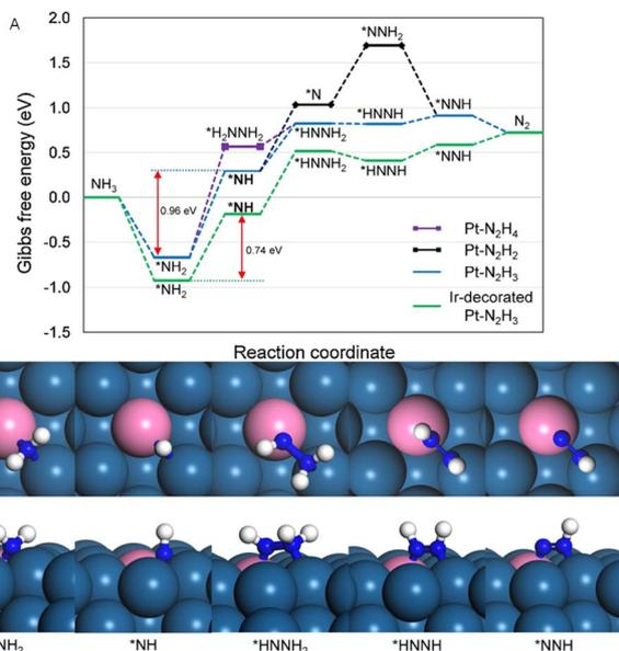
Fig. 9 (A) Gibbs free energy curves for AOR pathways on Pt(100) and Ir-decorated Pt(100) and (B) optimized structures (top and side views) of reaction intermediates using the N<sub>2</sub>H<sub>3</sub> route during AOR on Ir-decorated Pt(100). Color code: Ir, pink; Pt, dark blue; H, white; N, blue. Reproduced from ref. 9 with permission from Springer, copyright 2020.
