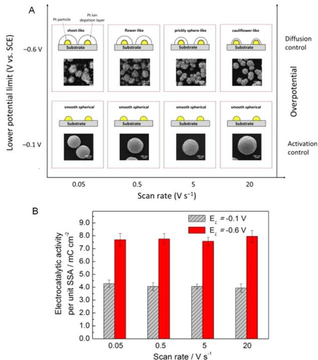
Fig. 8 (A) Schematic representation of a two-dimensional map illustrating how the voltage difference and scan rate affect the particle morphologies; and (B) Pt particles with varied morphologies and EL values of  $-0.1 \text{ V}$  and  $-0.6 \text{ V}$  have varying electrocatalytic activity per unit SSA. Reproduced from ref. 37 with permission from Elsevier, copyright 2013.
