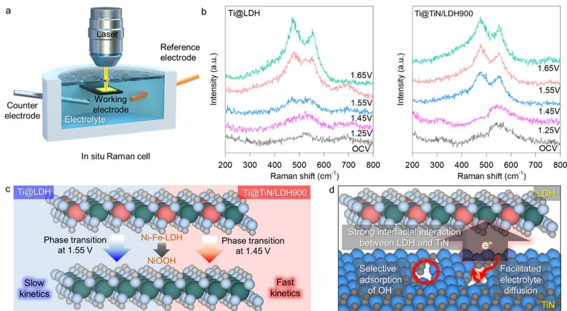
Fig. 5 (a) Instrumental setting for *in situ* Raman analysis. (b) *In situ* Raman data during the OER for Ti@TiN/LDH900 and Ti@LDH. (c) Impact of the TiN buffer layer on the phase transition behavior of anchored Ni–Fe–LDH species. (d) Scheme for efficient electronic coupling between the LDH and TiN buffer layer.
