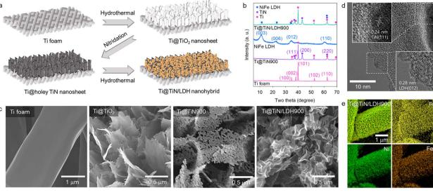
Fig. 1 (a) Scheme for the preparation of Ti@TiN/LDH foam. (b) Powder XRD, (c) FE-SEM, (d) TEM, and (e) EDS-mapping data of Ti@TiN/LDH nanohybrids and several references.
