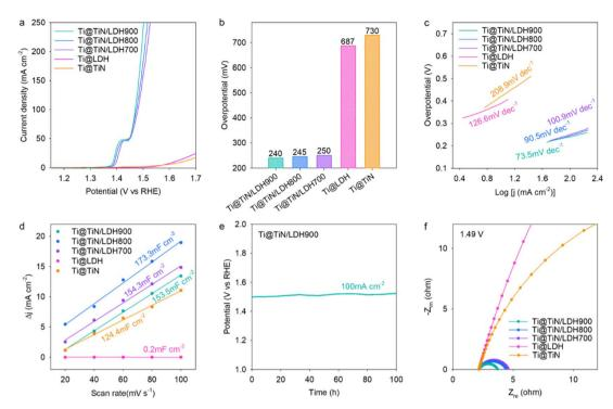
Fig. 3 (a) LSV of the OER with *iR* correction, (b) overpotentials, (c) Tafel slopes, (d) ECSA, (e) durability, and (f) EIS data of Ti@TiN/LDH700–900 measured in 1 M KOH electrolyte.
