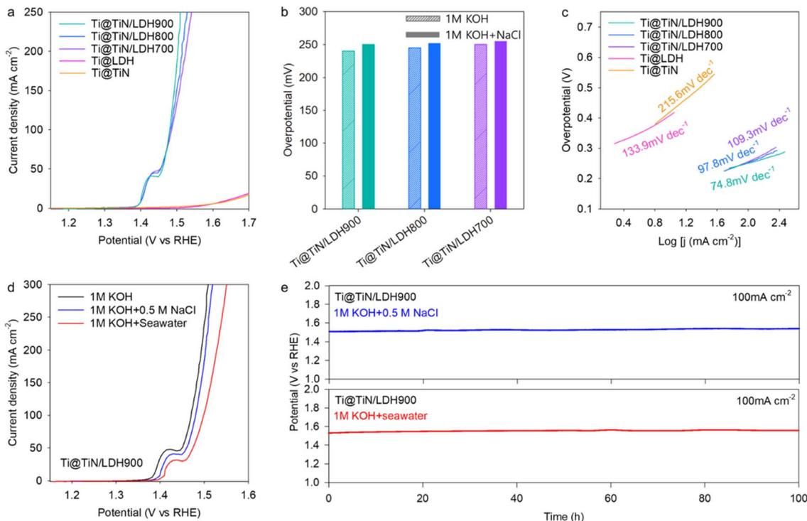
Fig. 4 (a) LSV of the OER with  $iR$  correction, (b) overpotentials, and (c) Tafel slopes measured in simulated seawater (i.e., 1 M KOH + 0.5 M NaCl) electrolyte. (d) Comparison of LSV data with  $iR$  correction and (e) durability data of Ti@TiN/LDH900 measured in simulated seawater and real seawater electrolytes.
