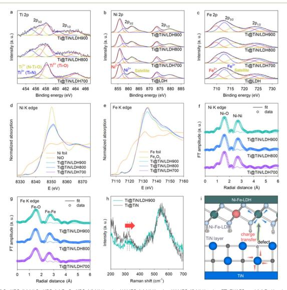
Fig. 2 (a) Ti 2p XPS, (b) Ni 2p XPS, (c) Fe 2p XPS, (d) Ni K-edge XANES, (e) Ni K-edge XANES, (f) Ni K-edge FT-EXAFS, and (g) Fe K-edge FT-EXAFS, and (h) micro-Raman data. (i) Schematic illustration for interfacial coordination between holey TiN and Ni-Fe-LDH.
