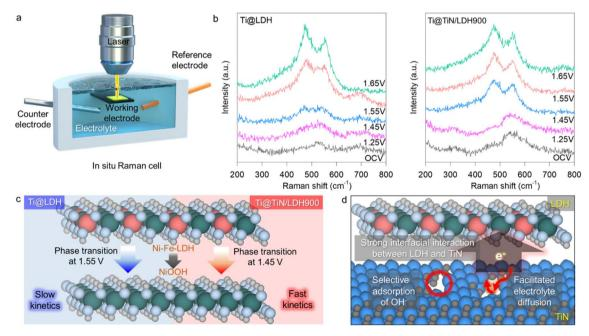
Fig. 5 (a) Instrumental setting for *in situ* Raman analysis. (b) *In situ* Raman data during the OER for Ti@TiN/LDH900 and Ti@LDH. (c) Impact of the TiN buffer layer on the phase transition behavior of anchored Ni–Fe-LDH species. (d) Scheme for efficient electronic coupling between the LDH and TiN buffer layer.
