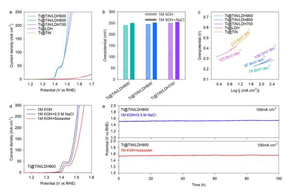
Fig. 4 (a) LSV of the OER with iR correction, (b) overpotentials, and (c) Tafel slopes measured in simulated seawater (i.e., 1 M KOH + 0.5 M NaCl) electrolyte. (d) Comparison of LSV data with iR correction and (e) durability data of Ti@TiN/LDH900 measured in simulated seawater and real seawater electrolytes.
