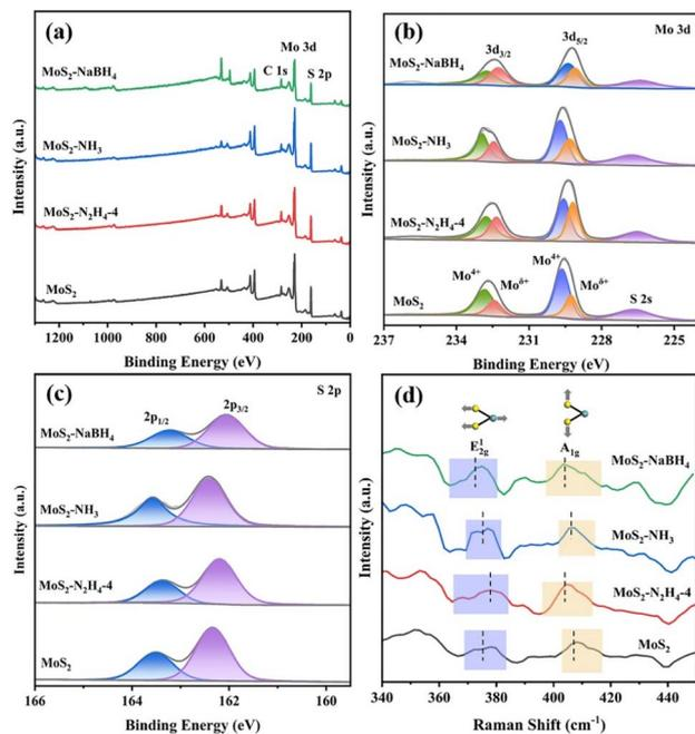
Fig. 3 (a) The XPS survey spectra and XPS spectra of (b) Mo 3d and (c) S 2p states in MoS<sub>2</sub>, MoS<sub>2</sub>-N<sub>2</sub>H<sub>4</sub>-4, MoS<sub>2</sub>-NH<sub>3</sub> and MoS<sub>2</sub>-NaBH<sub>4</sub> catalysts. (d) Raman spectra of MoS<sub>2</sub>, MoS<sub>2</sub>-N<sub>2</sub>H<sub>4</sub>-4, MoS<sub>2</sub>-NH<sub>3</sub> and MoS<sub>2</sub>-NaBH<sub>4</sub> catalysts.
