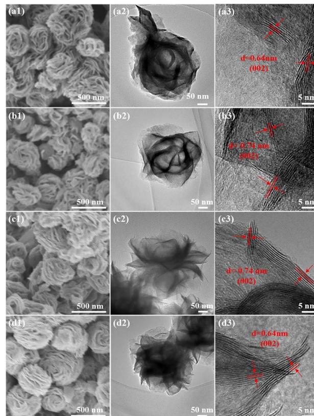
Fig. 2 (a1–d1) SEM, (a2–d2) TEM and (a3–d3) HRTEM images of (a1–a3) MoS<sub>2</sub>, (b1–b3) MoS<sub>2</sub>-N<sub>2</sub>H<sub>4</sub>-4, (c1–c3) MoS<sub>2</sub>-NH<sub>3</sub> and (d1–d3) MoS<sub>2</sub>-NaBH<sub>4</sub> catalysts.
