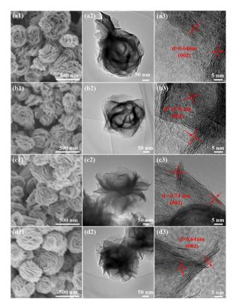
Fig. 2 (a1-d1) SEM, (a2-d2) TEM and (a3-d3) HRTEM images of (a1a3)  $MoS_2$ , (b1-b3)  $MoS_2-N_2H_4-4$ , (c1-c3)  $MoS_2-NH_3$  and (d1-d3) MoS<sub>2</sub>-NaBH<sub>4</sub> catalysts.
