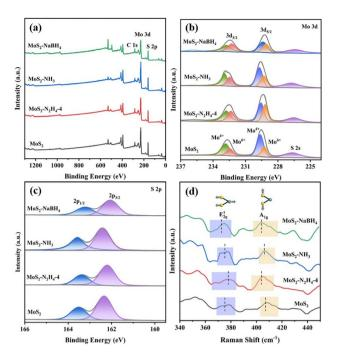
Fig. 3 (a) The XPS survey spectra and XPS spectra of (b) Mo 3d and (c) S 2p states in MoS $_2$ -N $_2$ H $_4$ -4, MoS $_2$ -NH $_3$  and MoS $_2$ -NaBH $_4$  catalysts. (d) Raman spectra of MoS $_2$ , MoS $_2$ -N $_2$ H $_4$ -4, MoS $_2$ -NH $_3$  and MoS $_2$ -NaBH $_4$  catalysts.
