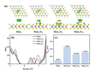
Fig. 6 (a) DFT calculated charge density difference diagrams of CO<sub>2</sub> adsorption, (b) total density of states, and (c) adsorption energy ( $E_{ads}$ ) of
