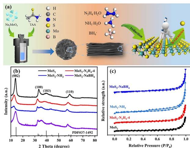
Fig. 1 (a) Sketch of preparation of  $\text{MoS}_2$  with varying interlayer spacing and Sv concentrations via the chemical reduction method. (b) XRD patterns and (c)  $\text{N}_2$  adsorption–desorption isotherms of  $\text{MoS}_2$ ,  $\text{MoS}_2\text{-N}_2\text{H}_4\text{-4}$ ,  $\text{MoS}_2\text{-NH}_3$  and  $\text{MoS}_2\text{-NaBH}_4$  catalysts.
