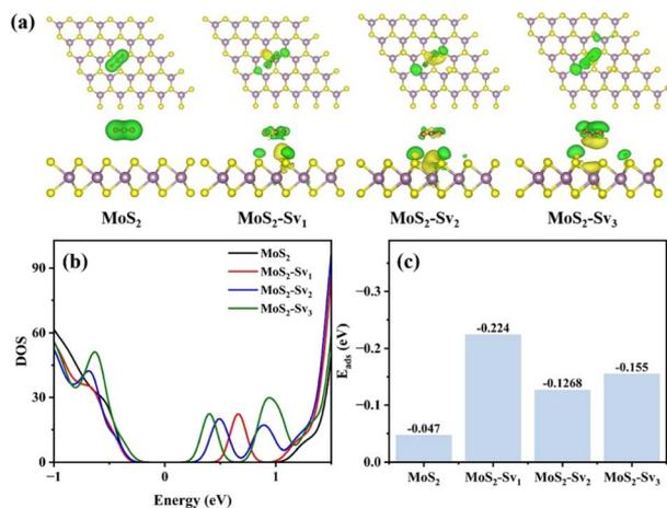
Fig. 6 (a) DFT calculated charge density difference diagrams of CO<sub>2</sub> adsorption, (b) total density of states, and (c) adsorption energy ( $E_{\text{ads}}$ ) of CO<sub>2</sub>.
