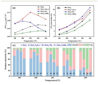
Fig. 4 (a) STY of CH<sub>3</sub>OH and (b) CO<sub>2</sub> conversion on MoS<sub>2</sub>, MoS<sub>2</sub>-N<sub>2</sub>H<sub>4</sub>-4, MoS<sub>2</sub>-NH<sub>3</sub> and MoS<sub>2</sub>-NaBH<sub>4</sub> catalysts. (c) Product selectivity of  $MoS_2$ ,  $MoS_2-N_2H_4-4$ ,  $MoS_2-NH_3$  and  $MoS_2-NaBH_4$  catalysts. Reaction conditions:  $V_{CO_2/H_2} = 1/3$ , GHSV = 8000 mL  $g_{cat}$ = 4.0 MPa.
