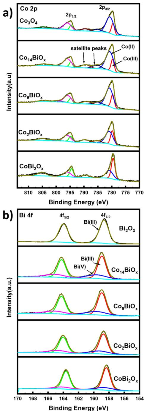
Fig. 4 High resolution XPS spectra showing peaks corresponding to (a) Co 2p and (b) Bi 4f of Co<sub>3</sub>O<sub>4</sub>, Co<sub>14</sub>BiO<sub>x</sub>, Co<sub>9</sub>BiO<sub>x</sub>, Co<sub>2</sub>BiO<sub>x</sub>, CoBi<sub>2</sub>O<sub>x</sub>, and Bi<sub>2</sub>O<sub>3</sub> catalysts.
