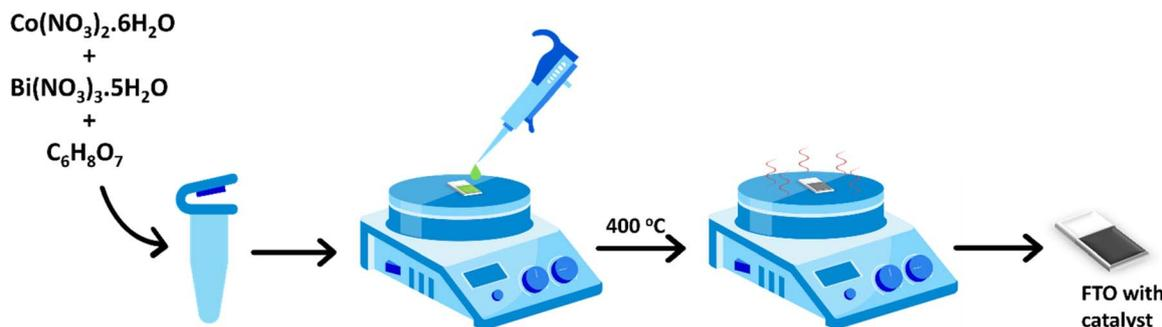
Fig. 1 Schematic of the synthesis of  $\text{Co}_2\text{BiO}_x$  catalysts on FTO. The procedure involves: (i) mixing Co(II) nitrate and Bi(III) nitrate in citric acid solution, (ii) deposition of the solution onto FTO substrate, and (iii) drying and annealing the FTO-deposited metal salts.
